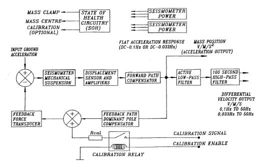
In comparison to a conventional feedback accelerometer the hybrid velocity response is obtained with a dominant single pole which is set at either 0.1 Hz or at 0.033 Hz. The dominant pole breaks the system response into two sections, the first one being flat to acceleration from dc to the dominant corner frequency (0.1 Hz or 0.033 Hz) and the second response flat to velocity starting from the dominant corner frequency until the high frequency cut off.
