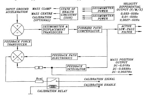
The system velocity responses are defined by a transfer function identical to that of a conventional long period sensor with a velocity transducer whose natural resonant frequency is set at 0.033 Hz, 0.01 Hz or 0.0027 Hz and the damping z at 0.707.
