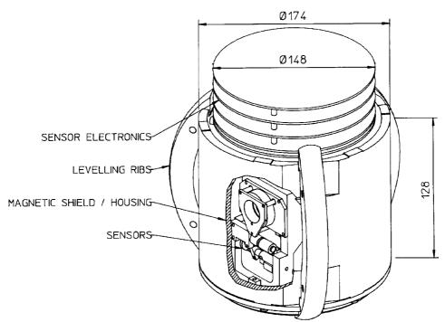
The levelling dish structure has  $\pm$  30 degrees of levelling capability, with an accuracy of  $\pm$  0.2 degrees, and stability which is fit to be used as a levelling platform for a broadband sensor.
