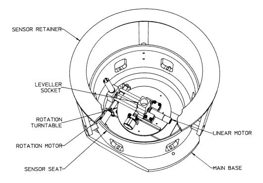
Two sets of position sensors fitted to the motor shafts transmit the digital shaft position signals to a micro-processor to enable precise radial and azimuth movement without slippage. In fact, the position detectors are absolute and provide position information without losing information when the system is switched off.
