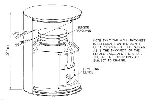
The positions of the mounting notes are given in the following drawings together with a suggested method of electrically isolating the levelling system from it's casing.
