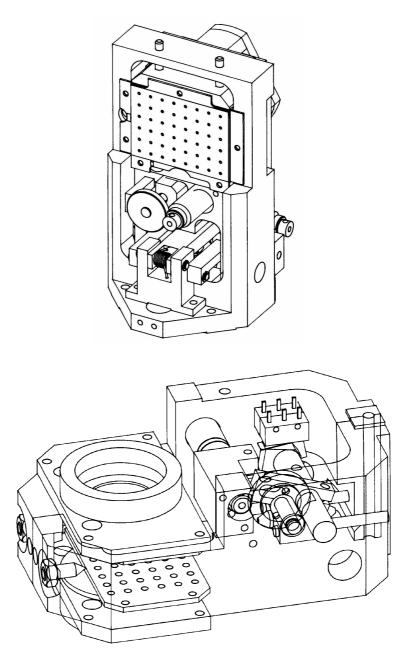
The adjustments required for operation consist of levelling the boom of the vertical sensor and tilting the bases of the horizontal sensors to centre the movements in their equilibrium positions. These adjustments are made by small DC motors operating through gear trains to tilt the bases of the horizontal sensors and to apply a small extra force to the vertical sensor's boom.
