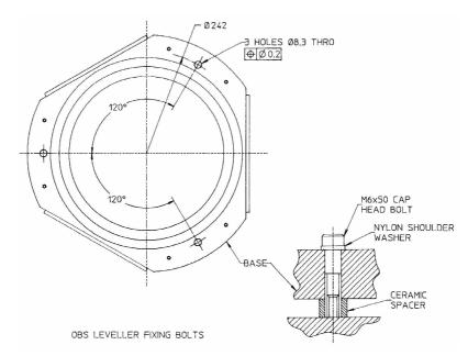
It is recommended that ceramic spacers with nylon shoulder washers are used to achieve a very high degree of insulation resistance,  $>>100M\Omega$ .
