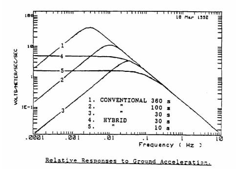
Alternatively the system amplitude plots are given below as output against input velocity.
