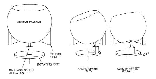
The described mechanism is more stable and more compact than the more usual gimbal arrangement and also has fewer moving parts. For broadband OBS seismometer applications the gimbal arrangement would not be sufficiently stable.
