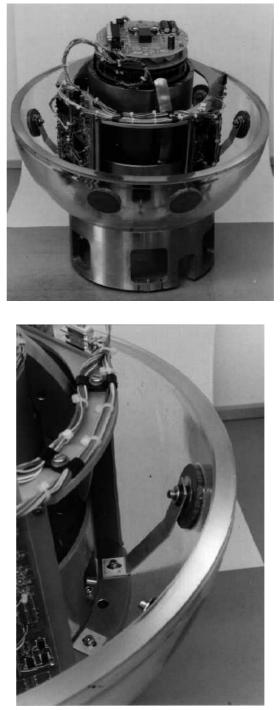
A set of attachment points are glued to the inside of the glass sphere from which semi-flexible linkages are used to attach the bottom of the levelling platform to the glass sphere. Six separate holes are provided for such linkages.
