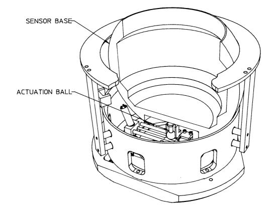
Individually each sensors outputs can be further zeroes within a range of  $\pm 2.5$  degrees. The horizontal sensors are levelled (or mass position output zeroed) by tilting the sensor bases, in the case of the vertical sensor the sensor boom position is controlled by the movement of the tip of the main load bearing spring.
