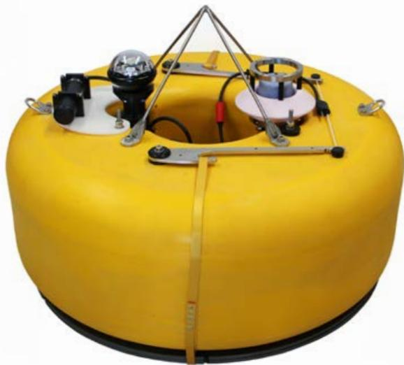
Compact, free-fall ocean-bottom seismometer with multi-disciplinary research capabilities and optional features for earthquake or tsunami early warning, without cables.
