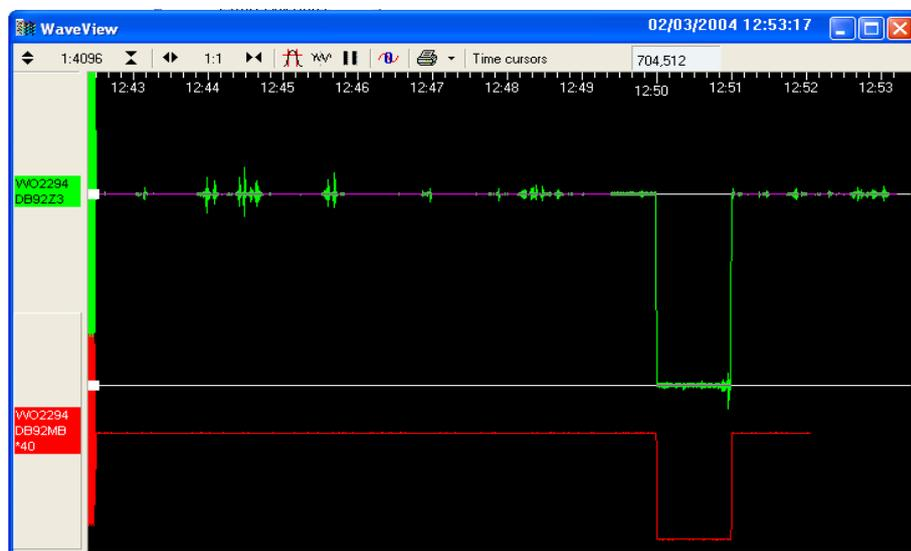
The **Ampl Cursors** button will now be displaying a value, which is the strength of the returning signal in counts (doubled, if using a sine wave). Measure the other two signal strengths in this manner.
