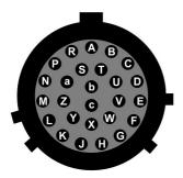
Wiring details for the compatible socket, \*\*\*-16-26S, as seen from the cable end.
