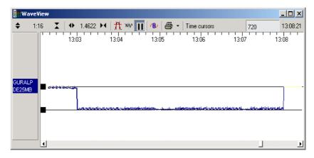
The **Ampl Cursors** button will now be displaying a value, which is the strength of the returned signal in counts (doubled, if using a sine wave). Measure the other two signal strengths in the same manner.
