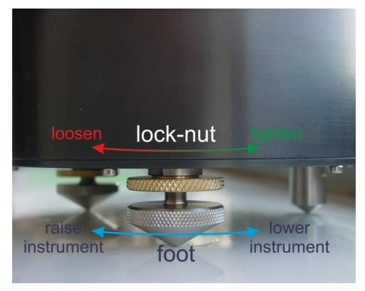
The instrument can use internal simulated level adjustment to compensate for tilt, as long as it is fixed within 1 ° of the horizontal.
