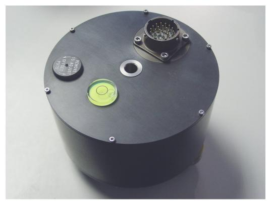
The 5T Compact system combines low-noise components with high feedback loop gain to provide a linear, precision transducer with a very large dynamic range. In order to exploit the entire dynamic range, two separate outputs - high and low gain are provided. Nominally, the high gain outputs are set to output a signal 10 times stronger than the low gain outputs.
