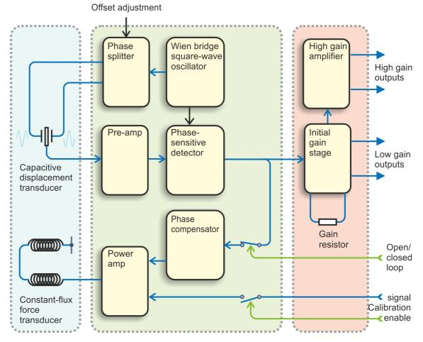
The mass and the capacitor plates are energised by a two-phase transformer driver, forming a differential capacitor. This acts as a capacitive transducer, whose signal is
