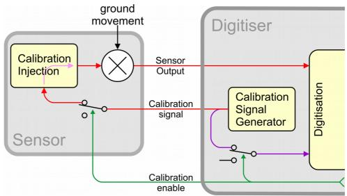
In this diagram, a Güralp digitizer is being used to inject a calibration signal into the sensor. This can be either a sine wave, a step function or broad-band noise,
