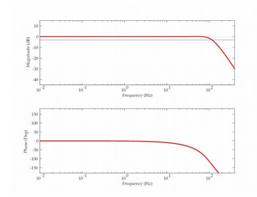
When testing the instrument to confirm that it meets its design specification, the range of frequencies used are concentrated over about 3 decades (*i.e.* 1000 : 1) of excitation frequencies. Consequently, the frequency plots of each component are provided in normalised form. Each plot marks the frequency cut-off value (often quoted as "-3 dB" or "half-power" point).
