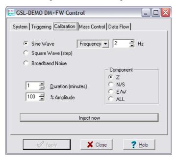
2. Select the calibration channel corresponding to the instrument, and choose **Broadband Noise.** Select a suitable duration and amplitude, and click **Inject now**. A new data stream, ending  $C\underline{n}$  ( $\underline{n} = 0 - 7$ ) or MB, should appear in Scream!'s main window containing the returned calibration signal.
