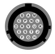
Wiring details for the compatible plug, \*\*\*-14-19P, as seen from the cable end (*i.e.* when assembling).
