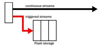
Instructs the digitizer to transmit any *continuous* streams directly to clients as for *DIRECT* mode, but to store *triggered* data into Flash storage as for *FILING* mode.
