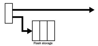
Instructs the DM24 to transmit streams directly to clients as for DIRECT mode, but also to store all data into Flash storage as for FILING mode. If a client fails to acknowledge a block, the digitizer does not attempt to retransmit it.
