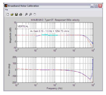
The accuracy of the results depends on both the amount of data you have selected and on its sample rate. To obtain good-quality results at low frequency, it will save computation time to use data collected at a lower sample rate; although the same information is present in higher-rate streams, they also include a large amount of high-frequency data which may not be relevant to your purposes.
