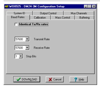
This tab allows the setting of the line speed for the main serial output.
