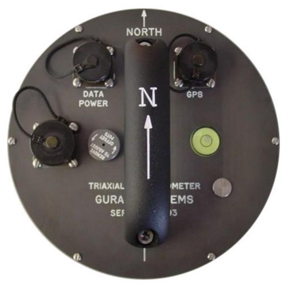
It is provided with a combination baseplate/mounting plate, which is separable and re-attachable, allowing for quick installation/removal and sensor site re-occupation if necessary. The DC offsets are available at the analogue output connector of the CMG-5TD and are user-accessible and adjustable via adjusting screws on the top cap of the instrument. A GPS receiver is used to provide accurate time-stamps for seismic data. The GPS receiver is attached to the CMG-5TD via a supplied 20 metre cable.
