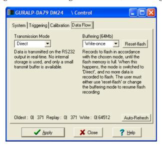
To choose a transmission or buffering mode, choose options from the *Transmission Mode* or *Buffering* drop-down menus, and click **Apply**. An explanation of the chosen mode is displayed beneath each menu. The following sections also explain the filing modes available.
