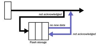
Instructs the digitizer to transmit current blocks to clients if possible, but to store all unacknowledged blocks in the Flash memory and re-send them, oldest first, when time allows. *ADAPTIVE* mode is best suited for "real-time" installations where the link between digitizer and client is intermittent or difficult of access.
