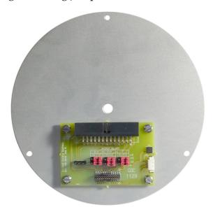
Each component (vertical, North/South and East/West) has two associated jumpers (one for each leg of the differential connection) and these must always be moved in pairs. It is possible to select different gains for different channels but this is rarely desirable. Consult the markings on the printed circuit board and the pictures below to select the desired gain.
