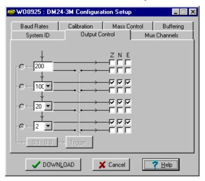
**Stream selection**: The digitiser has three channels or streams. These are depicted by the three columns labelled Z, N and E in the Output Control window shown above.
