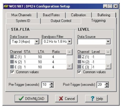
The Data Source button selects the tap (streams) that will be evaluated for triggers for both the STA/LTA and the Level triggers. In general, it is not
