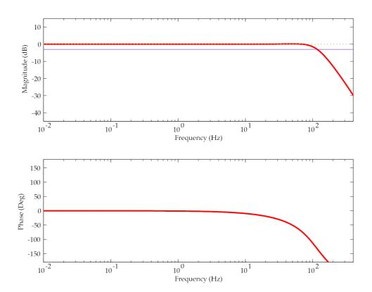
If you want to repeat the calibration to obtain more precise values at a particular frequency of interest, or to check that a sensor is still functioning correctly, you can inject calibration signals into the system using a Güralp digitizer or your own signal generator, and record the instrument's response.
