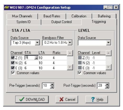
**Level triggering parameters**: The user specifies the Data Source, channels and levels by clicking on them, similar to the STA/LTA settings. The levels are specified in counts.
