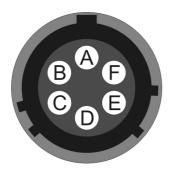
Wiring details for the compatible plug, \*\*\*-10-06P, as seen from the cable end (i.e. during assembly).
