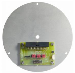
Each component (vertical, North/South and East/West) has two associated jumpers (one for each leg of the differential connection) and these must always be moved in pairs. It is possible to select different gains for different channels but this is rarely desirable. Consult the markings on the printed circuit board and the pictures below to select the desired gain:
