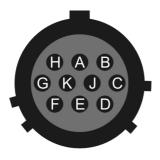
Wiring details for the compatible socket, \*\*\*-12-105, as seen from the cable end (*i.e.* when assembling).
