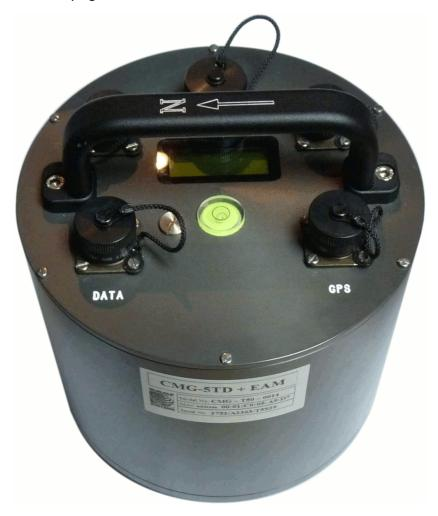
Full-scale low-gain sensitivity is available from 4.0 g down to 0.1 g. The most common configuration is for the 5T unit to output 5 V single-ended output for 1 g ( $\approx$  9.81 ms<sup>-2</sup>) input acceleration. The standard frequency pass-band is flat to acceleration from DC to 100 Hz (although other low pass corners can be ordered.) A high frequency option provides flat response from DC to 200 Hz.
