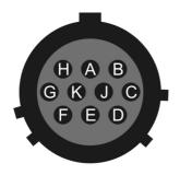
Wiring details for the compatible socket, \*\*\*-12-10S, as seen from the cable end (i.e. during assembly).
