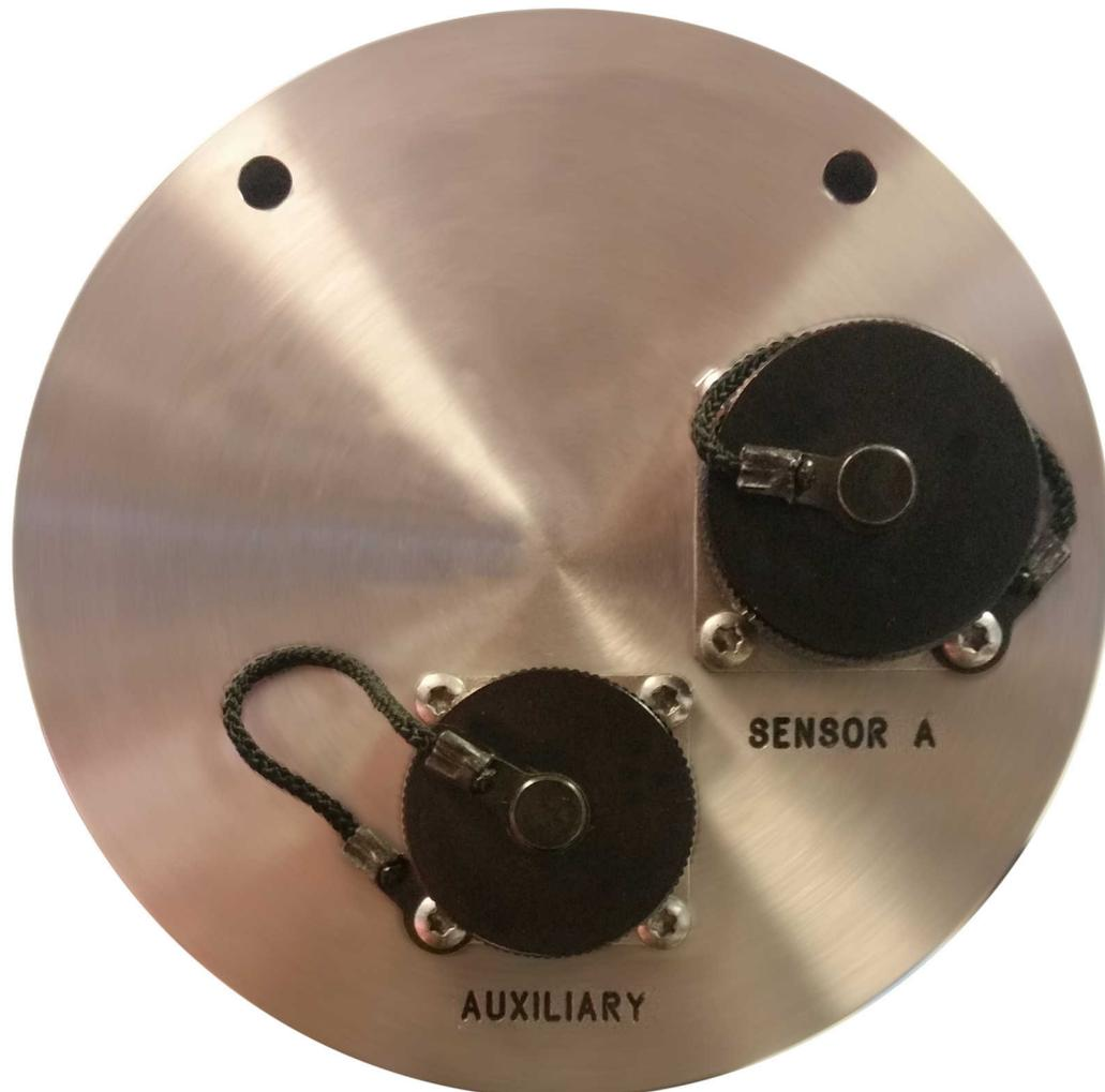
The analogue connector panel of the Affinity has one or two SENSOR connectors (depending on the model) and an AUXILIARY connector. The pin-outs for these connectors are given in the following sections.
