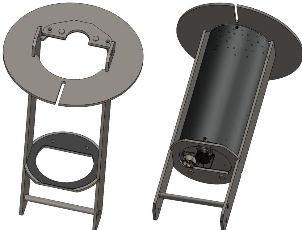
5. Feed the free end of the signal cable up through the hanger frame. It should pass the bar at the bottom of the hanger on the side towards the straight edge of the hole in the lower plate.
