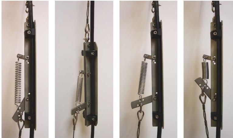
8. Fix the signal cable to the main lifting cable about one meter above the strain relief mechanism using a cable clamp (a nylon cable tie may be sufficient for shallow installations). Leave a little slack in the signal cable between the clamp and the strain relief mechanism.
