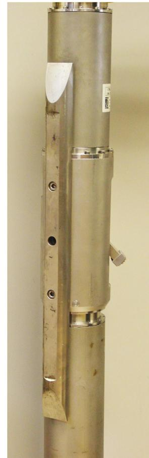
Studs have the advantage of being smaller than skids, but the contact points are very close to each other. You should evaluate the various locking methods available to see which works best in your borehole.
