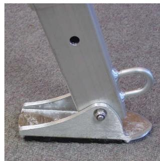
3. Erect the tripod above the borehole, and run the yellow retaining tape through the loops. Fasten together the ends of the tape.
