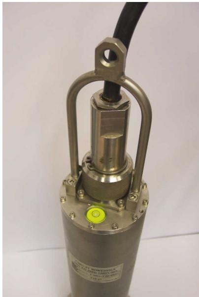
6. Join the loop to the bottom of the strain relief mechanism or surge-suppressor sonde using the linking cable provided.
