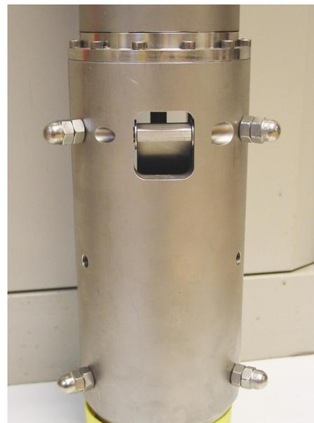
The motor has a power system separate from that of the sensor, and can be controlled from the surface using a hole lock control unit. Once the sonde is installed, the hole lock control unit may be removed. Without power, the hole lock will not be able to retract, and the sensor will be secured.
