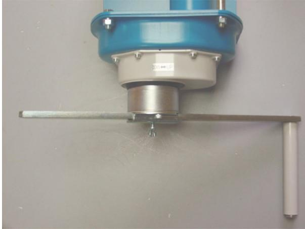
11. Hang the strain relief unit and instrument(s) from the loop at the other end of the cable. You are now ready to lower the assembly into the borehole as described above.
