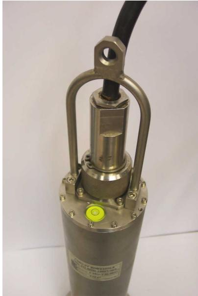
5. Join the loop to the bottom of the strain relief mechanism or surge-suppressor sonde using the linking cable provided.
