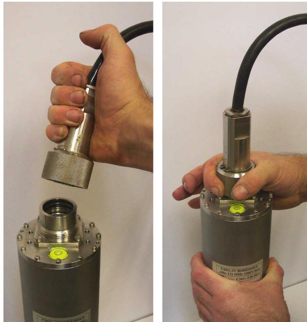
times during tightening in order to ensure that the connector is screwed fully home.
