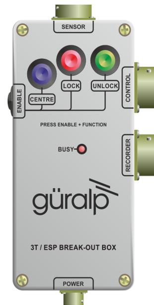
For deep-borehole installations (over 50 metres) may be necessary to use a modified instrument (with “active-high” logic ) and a breakout box with internal line drivers, to ensure that logic signals are reliably transmitted to the sensor. Contact Güralp Systems for advice.
