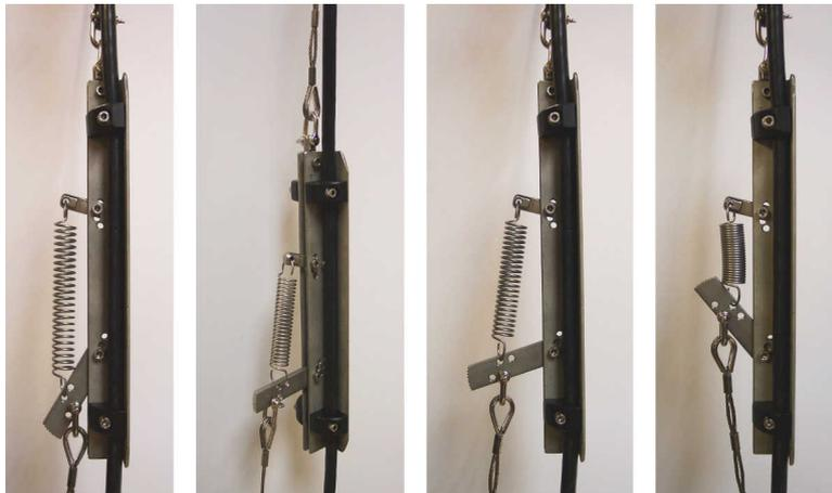
7. Fix the signal cable to the main lifting cable about one metre above the strain relief mechanism using a cable clamp (a nylon cable tie may be sufficient for shallow installations). Leave a little slack in the signal cable between the clamp and the strain relief mechanism.
