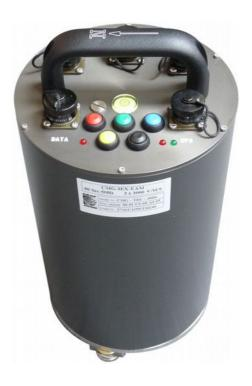
Each seismometer is delivered with a detailed calibration sheet showing its serial number, measured frequency response in both the long period and the short period sections of the seismic spectrum, sensor DC calibration levels, and the transfer function in poles/zeros notation.
