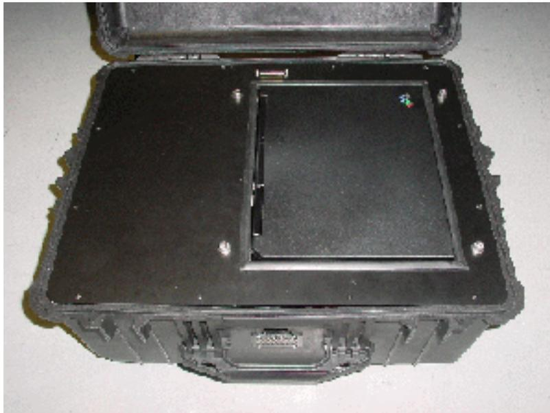
The housing of the digitiser is made from high impact copolymer polypropylene with mil-spec connectors fitted on to metal plates. There is also a small internal pocket for storing cables or documentation. The unit features a roller trolley design for ease of transportation.
