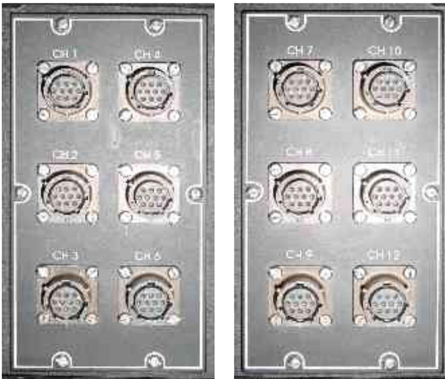
The DM24S12AMS unit's 12 analogue input connections are each identical to the output connection of the Güralp CMG-5U. These connections also serve as the sensors' 12V power supply. If required, other types of sensor may also be wired to a DM24S12AMS module.
