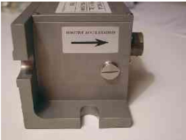
The 5U system combines low-noise components with high feedback loop gain to provide a linear, precision transducer with a very large
