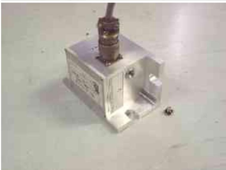
Although converting a sensor from horizontal to vertical response involves compensating for the acceleration due to gravity, you do not have to zero the sensor manually. The sensor output offset adjustment is carried out electronically by emulating the shift in mass position. You can then calibrate the offset using a potentiometer within the unit, without any loss of dynamic range.
