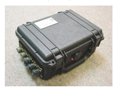
A stand-alone DCM unit is normally supplied with a high-capacity removable disk for data storage. These disks allow the DCM to be used as part of completely autonomous installation in cases where communications links are poor or non-existent. Manufactured and tested at Güralp Systems, the disks are compatible with USB and FireWire standards and include an internal temperature sensor and heater for use in cold environments.
