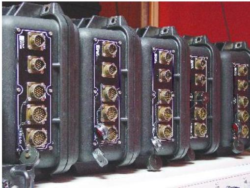
The CMG-DAS range of products combine the flagship CMG-DM24 analogue-to-digital converter with the communications, storage and protocol flexibility of the CMG-EAM in a single package.
