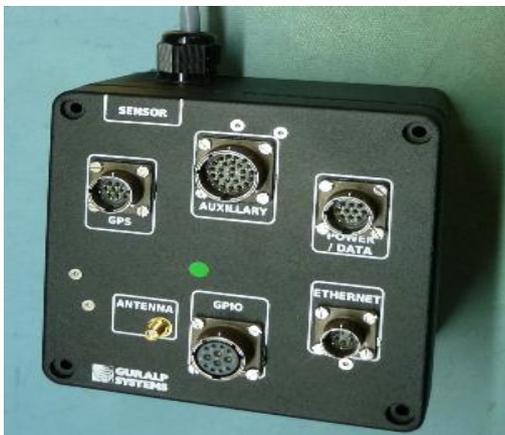
The CMG-EAM is available in a variety of packages including Peli-case (as shown above), borehole, ocean-bottom and metal tube (steel or aluminium) versions (top left).
