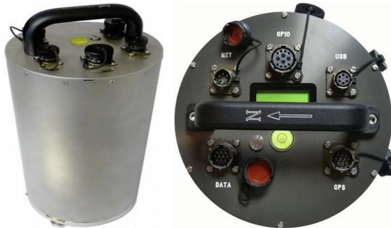
Integrated instruments (seismometer or accelerometer, digitiser and EAM)
