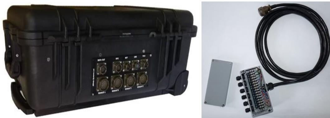
Each of the four breakout boxes has terminal connectors for up to 6 channels and connects to the DAS using 32 pin mil spec connectors.
