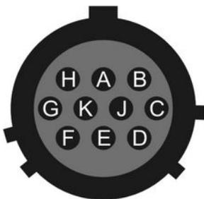
Wiring details for the compatible socket, \*\*\*-12-10S, as seen from the cable end (i.e. during assembly).
