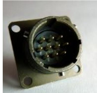
The pin-out is the same as the serial output of a DM24 digitizer, allowing you to insert a acquisition module into a pre-existing installation and maintain connectivity.
