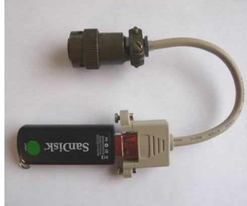
The adapter cable is required when upgrading the firmware of most acquisition module units but not when upgrading a CMG-NAM.
