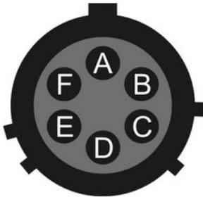
Wiring details for the compatible socket, \*\*\*-10-06S, as seen from the cable end (i.e. during assembly).
