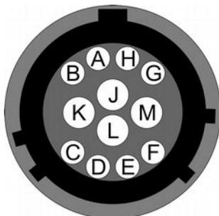
Wiring details for the compatible plug, \*\*\*-14-12P, as seen from the cable end (i.e. during assembly).
