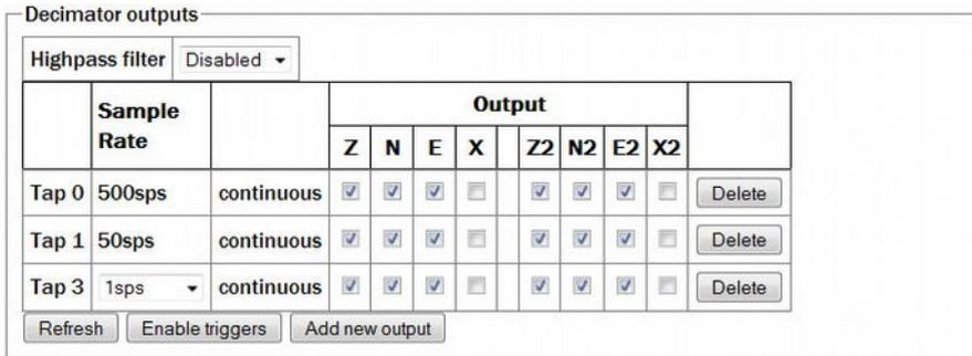
Streams from the second sensor are enabled or disabled by ticking or clearing the check-boxes in the columns labelled Z2, N2 and E2. An X2 stream will appear in this table when a seven- or eight-channel digitiser is detected, but it is not available on a seven-channel digitiser.
