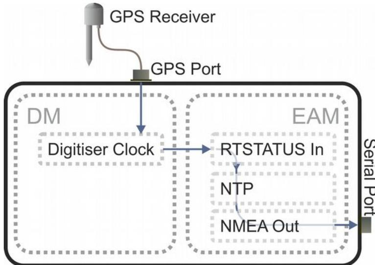
If required, the NTP subsystem can provide NMEA output via a serial port which can then be used to synchronise an additional digitiser. This, however, is optional and no serial port is dedicated to this use.
