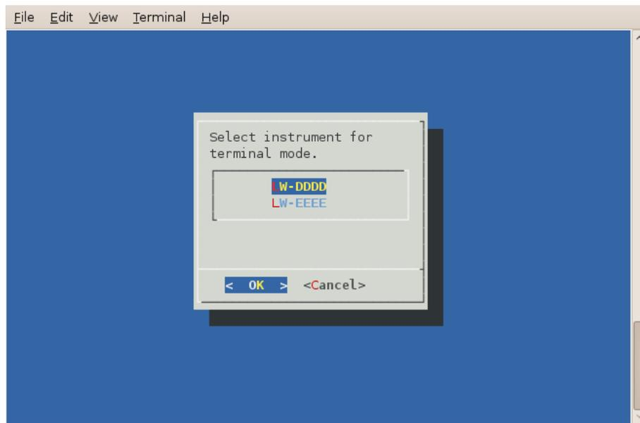
Select the required digitiser from the menu. The data-terminal program will suspend any service running on the associated port and start a minicom session with the correct communications parameters already set.
