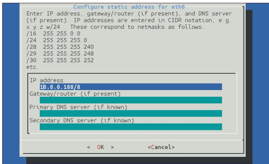
The IP address field must be populated with a valid IP address in CIDR notation. If you know the netmask but not the corresponding CIDR notation, use the information on screen as a guide or search the web for an on-line converter.
