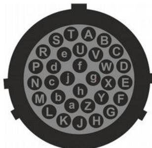
Wiring details for the compatible socket, \*\*\*-16-32S, as seen from the cable end (i.e. during assembly).
