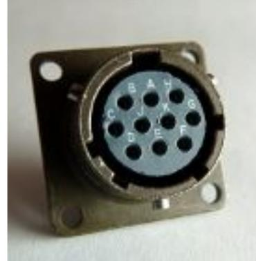
The pin-out is such that the port can be connected to the serial output of a DM24 digitizer using a straight-through cable.
