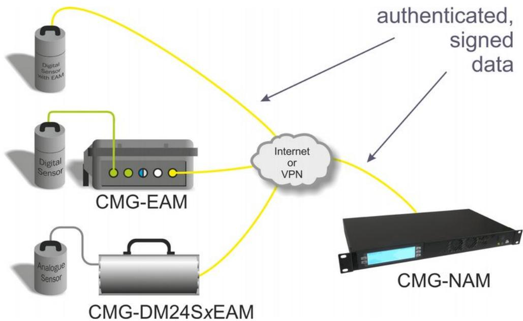
Platinum firmware has support for CD1.1 frame generation and forwarding with strong authentication provided by an optional embedded Spyrus hardware encryption device, allowing CMG-EAMs and CMG-NAMs to form the basis of a secure CD1.1 network.
