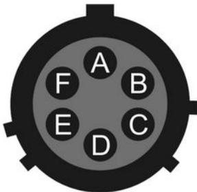
Wiring details for the compatible socket, \*\*\*-10-06S, as seen from the cable end (i.e. during assembly).
