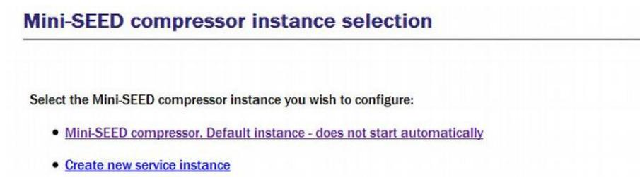
Although the default instance is marked as “does not start automatically”, it will be started if a dependant service is started.
