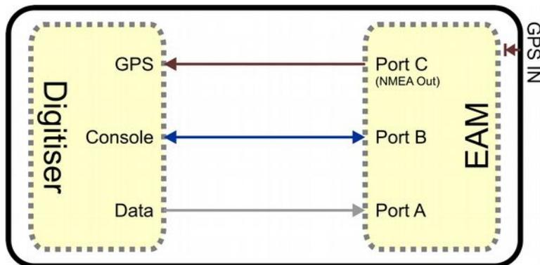
Both the digitiser's GPS input and Port C of the acquisition module must run at 4,800 Baud. This should never be changed. Note that, in this mode, the external GPS socket is disconnected: it cannot be used as an output for additional digitisers.
