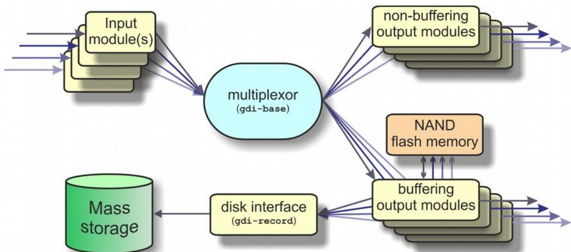
The multiplexor makes incoming data available to the output modules. These come in two flavours: simple modules (such as those for WIN, GSMS and QSCD) simply convert the data streams and output them in the required format; other modules maintain a ring-buffer which is used to, for example, satisfy BRP back-fill requests. The ring-buffers use the NAND flash memory. These output modules also send data to `gdi-record`, which handles all mass storage device writing requests, regardless of format.
