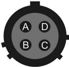
Wiring details for the compatible socket, \*\*\*-08-04S, as seen from the cable end (i.e. during assembly).
