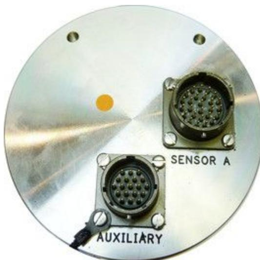
The illustration shows a four-channel unit; the seven-channel unit has an additional connector for sensor B:
