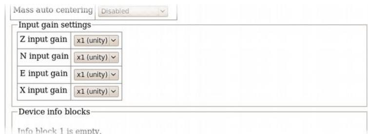
(This table is extended to show three additional components when a seven-channel digitiser is detected.)
