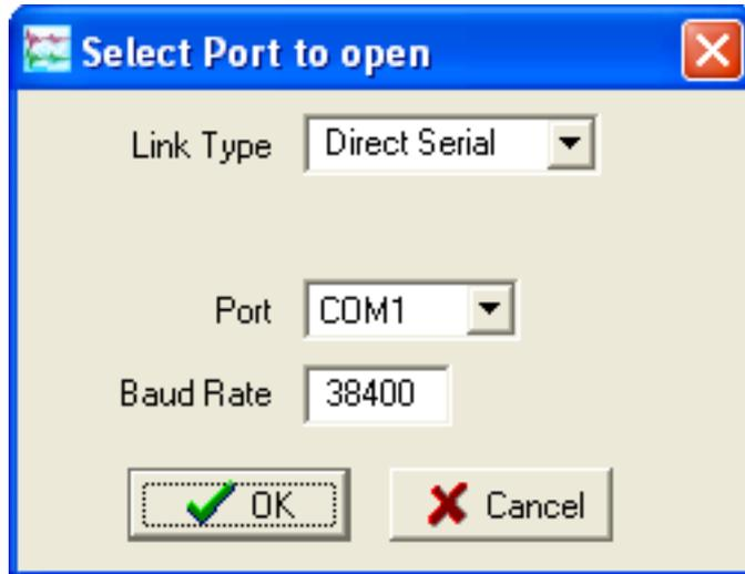
Set the Baud Rate to 38400, as shown, and, once the acquisition module and computer are communicating properly, an emulation window will open and you will see the **Login:** prompt. If it does not appear immediately, press the ENTER key a few times.
