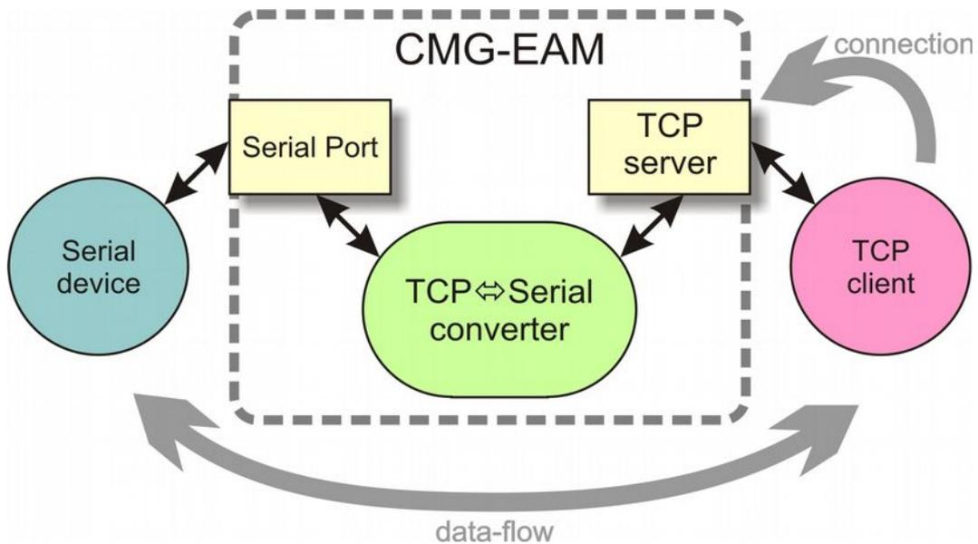
The acquisition module can be configured to only listen on particular addresses and ports, to only accept connections from certain addresses or blocks of addresses and to reject connections from certain addresses or blocks of addresses.
