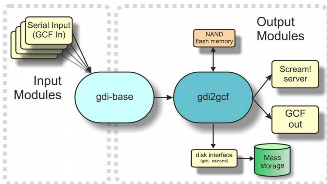
The `gdi2gcf` module, known as the GCF compressor, is responsible for re-blocking GDI samples into GCF blocks. It provides data to all GCF output modules as well as to the `gdi-record` module, which writes GCF files to the mass storage device. It has a number of configuration options, which are described in section 11.2 on page 138.
