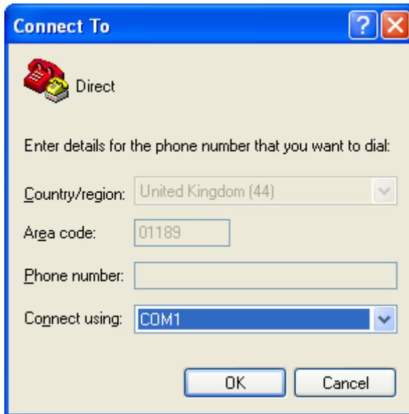
The **Country/region**, **Area code** and **Phone number** fields can be ignored: they are only used when working with modem connections. Select the name of the correct COM port from the **Connect using** drop-down menu, then click .
