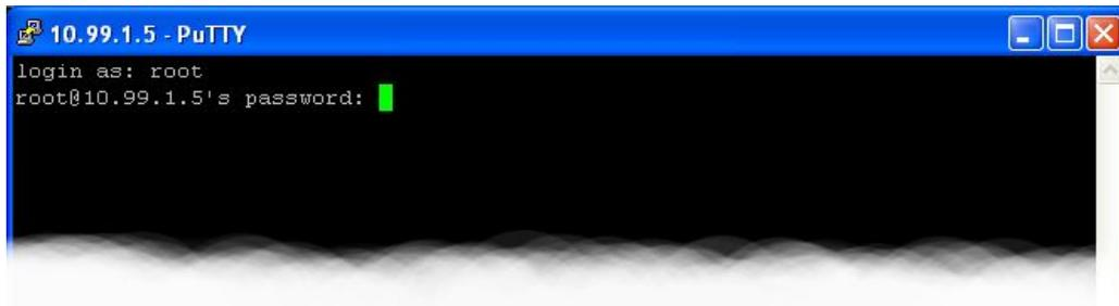
Once connected, you will be presented with a shell prompt which is ready to accept commands. The shell prompt contains the serial number of the acquisition module.
