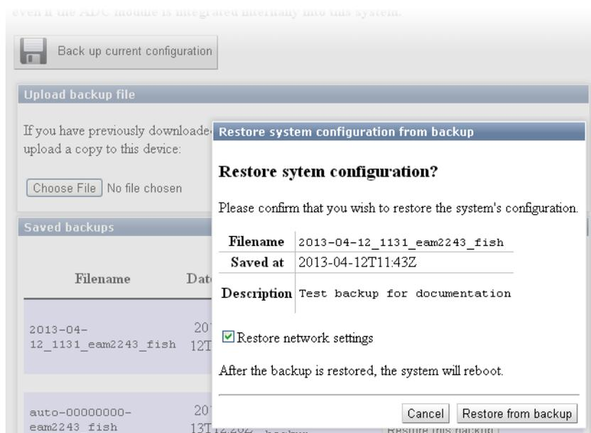
The date and time at which the backup was saved is shown; in the example above, this is the 12th of April, 2013 at 11:43. The file name and description of the backup are also given.
