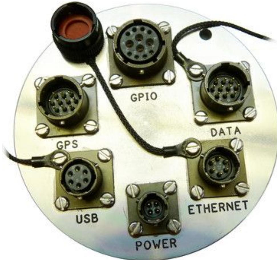
For more information on the ports see section 2.5 on page 14. The connector pin-outs are given in section 14.1.1 on page 218 and listed in the table below:
