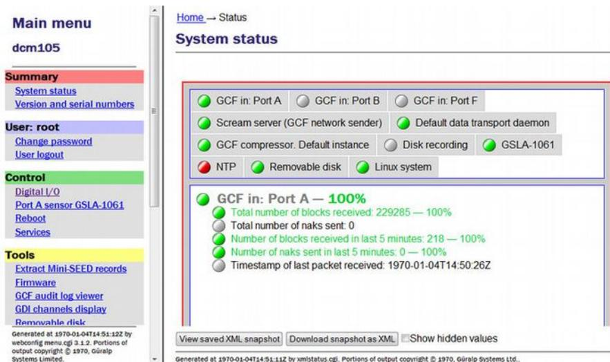
The left-hand frame contains the system ID above a menu while the main frame displays sub-menus, input forms and display screens.
