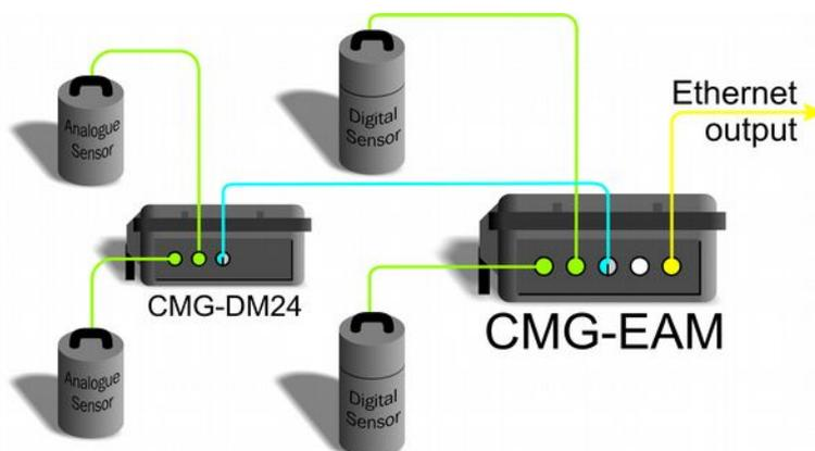
If the output link is over a network, all external serial ports of a standard CMG-EAM (including the “DATA OUT” port) are available for connection to digitisers or digital instruments, allowing up to eighteen channels to be aggregated. An arbitrary number of CMG-EAMs may be chained together, allowing for even more extensive arrangements.
