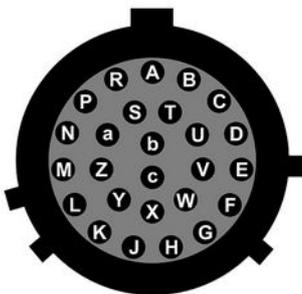
Wiring details for the compatible socket, \*\*\*-16-26S, as seen from the cable end (i.e. during assembly).
