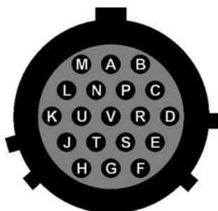
Wiring details for the compatible socket, \*\*\*-14-19S, as seen from the cable end (i.e. during assembly).
