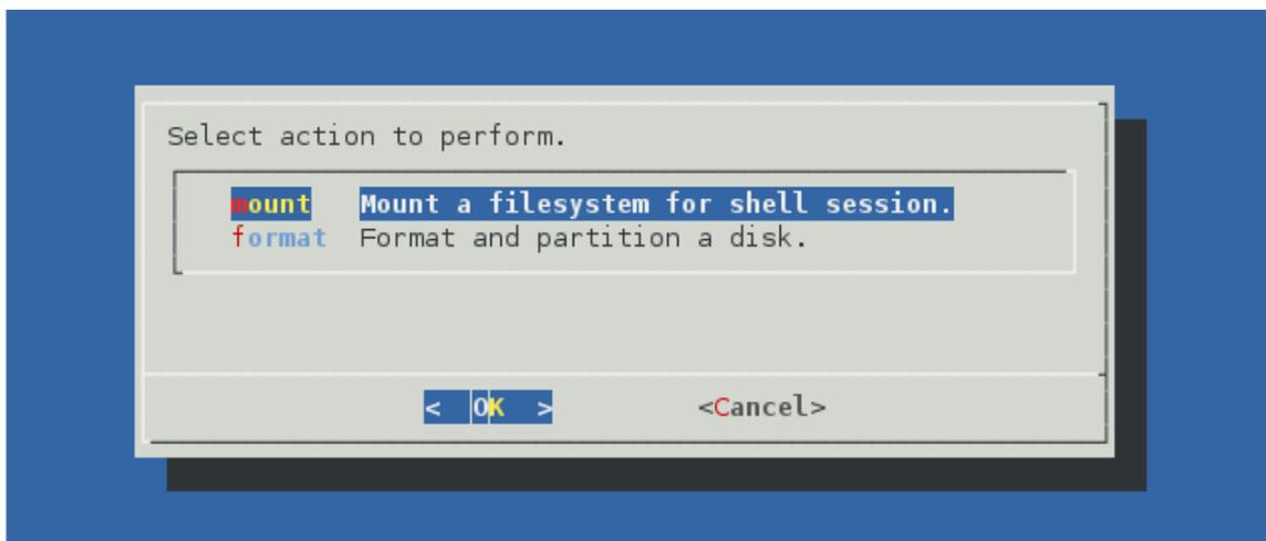
The “mount” option, which can be selected with the  key, displays a menu of available file-systems on removable media. When you choose your desired file-system, it is mounted under `/media` and you will be told the exact mount point and then presented with a command prompt. This is a sub-shell: the file-system will remain mounted and the mass storage device will remain
