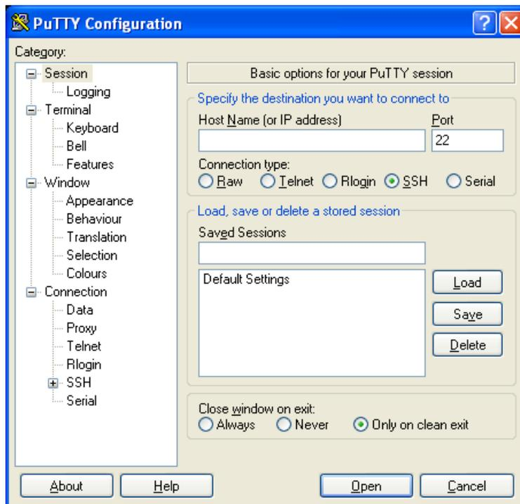
Enter the IP address of the acquisition module into the **Host Name (or IP address)** field, check that SSH is selected as the **Connection type** and then click the
