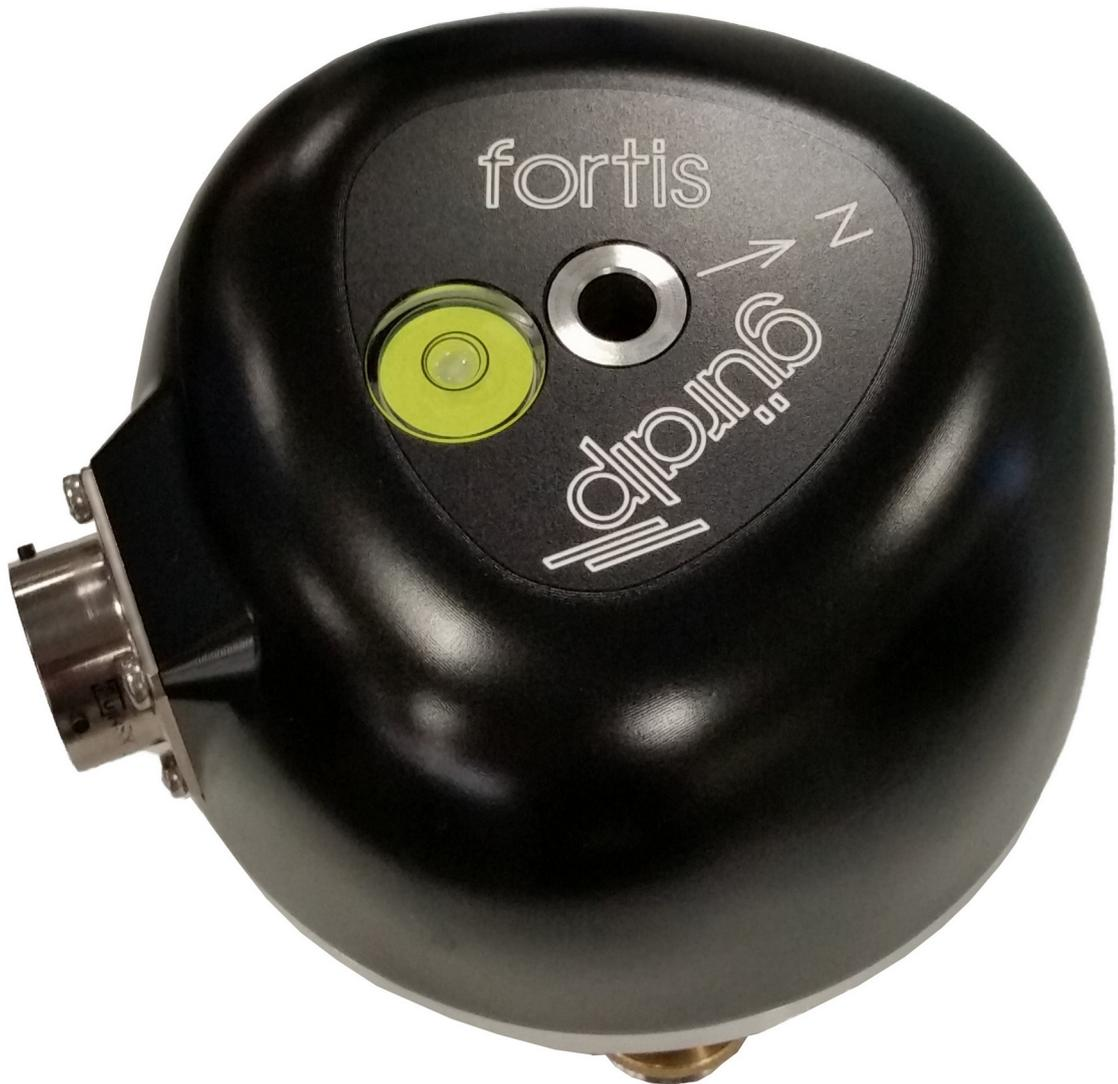
The hard-anodised aluminium casing protects the instrument from water, allowing it to be deployed in a range of environments. Installation is simple, using a single fixing bolt to attach the sensor to a hard surface. If required, you can also level the sensor using its adjustable levelling feet. An integrated bubble-level provides quick visual feedback.
