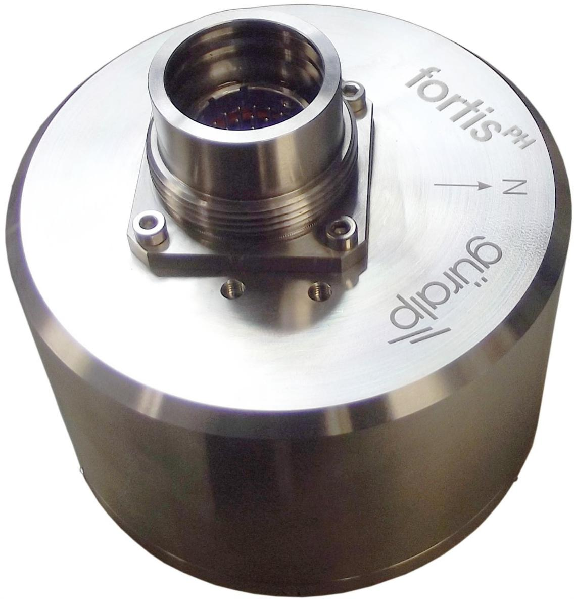
The Fortis accelerometer is also available in borehole-specific packaging. This variant is called the Fortis Post-hole, or Fortis<sup>PH</sup>. The components and electronics inside the sensor are identical to the surface module: the only difference is in the external casing and the connector, which is water-proof to 100 Bar (equivalent to 10 MPa or 1500 psi). See section 7.2 on page 32 for pin-out details.
