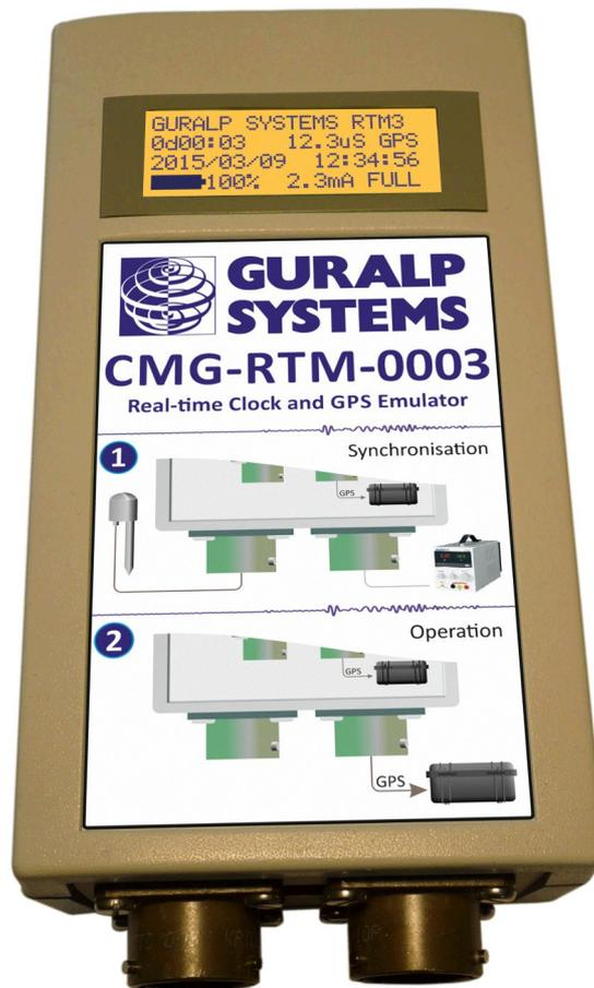
Once the initial synchronisation source is removed, the CMG-RTM continues to run under battery power, maintaining timing through the use of a high-precision, thermally-compensated, crystal-controlled oscillator. The CMG-RTM can then be transported to the deployment site and connected to a digitiser, from which it subsequently draws power. Once powered, it will generate the NMEA and PPS signals which are required to synchronise the connected digitiser.
