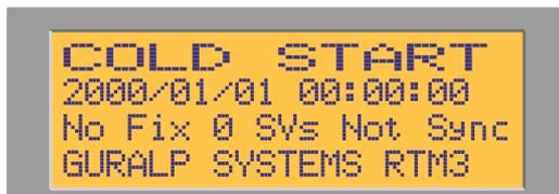
In the illustration above, the receiver does not know where it is (No Fix) and it can see no satellites (SVs stands for "Space Vehicles", which is standard GPS terminology for the satellites used by the GPS system). As a result, the system is not synchronised (Not Sync).
