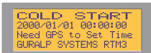
The second line shows the date and time, according to the internal clock. The third line shows that no GPS data are currently being received.
