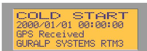
The GPS receiver produces two sets of outputs: a stream of textual data known as the NMEA (because it is in NMEA 0183v1.5 format) and a one-Hertz pulse train known as the PPS. The NMEA provides coarse timing (to the nearest second) and the PPS provides accurate sub-second timing.
