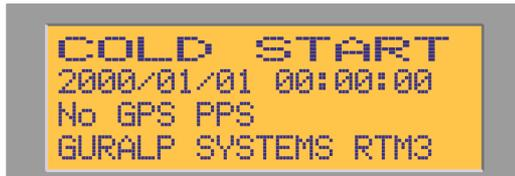
If you see either of these screens, please check the GPS cable and connections. If no fault is apparent, please contact GSL technical support for advice.
