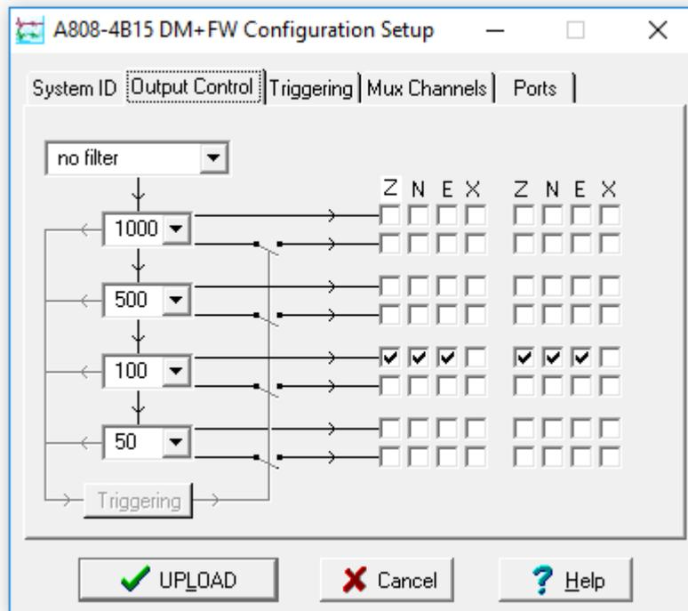
Güralp digitisers initially sample incoming data at a high rate (*e.g.* 2000 Hz for the DM24), which is then filtered and reduced to a lower rate (*decimated*) using an on-board digital signal processing unit, or DSP. The DSP has several filtering-decimation stages, which run one after the other. Stages which can produce output
