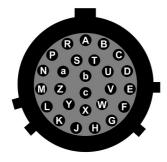
Wiring details for the compatible socket, \*\*\*-16-26S, as seen from the cable end (*i.e.* when assembling).
