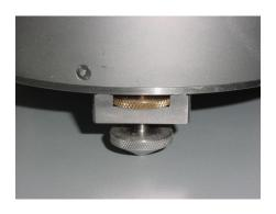
Loosen the brass locking nut on one of the adjustable feet. Turn the foot, screwing it in or out to level the sensor. Check using the spirit level on the sensor lid.
