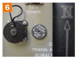
Remove the screw-on cap protecting the offset adjusters. With a small screwdriver, adjust each offset until the corresponding output in the waveview window is close to zero. Zoom in as necessary.
