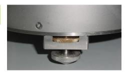
Loosen the brass locking nut on one of the adjustable feet.
