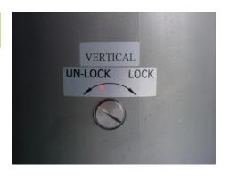
Remove the screw cap protecting the vertical lock access socket, and insert a hexaghonal wrench.. Find the retaining screw within, and loosen it to unlock the vertical component. Repeat for the north/south and east/west components.
