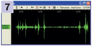
Run Scream! on a computer elsewhere on your network, and use the Network Control window to add a new UDP server at port 1567 of the EAM. Right-click and select GCFSEND: B. Check that the data streams appear.
