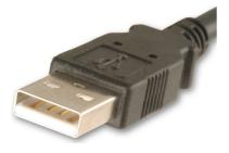
USB connections are very sensitive to wiring details so it is recommended that ready-made cables are used where possible. When used with a CD24-R8, Type A to Type B cables are required.
