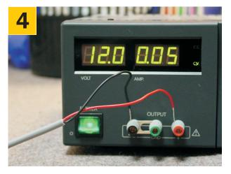
Switch on the power supply and measure the current through the instrument. Either
