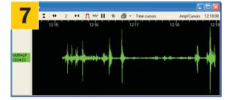
Select the *CD24Z2* data stream and double-click it. A *Waveview* window will open on the stream. Check that the output responds to vibrations near the sensor.
