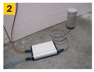
Choose suitable sites to install the sensor and GPS. The sensor should be placed
