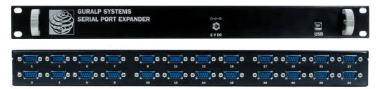
These systems have a single USB type B connector on the front panel and eight, sixteen or twenty-four nine-pin serial ports on the rear panel. Because the serial ports require more power than is available from a single USB connection, a 5 V DC power input is required.
