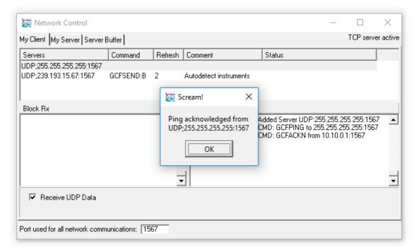
In this case, a single acknowledgement response (GCFACKN) was received and it came from the address 10.10.0.1 so this is the address of the NAM. If there are more than one NAM (or other GCF servers) on the network, multiple GCFACKN packets will be reported, as shown here:
