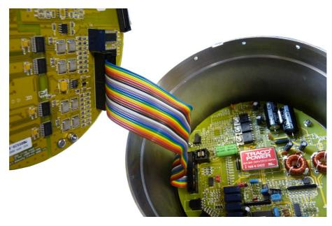
6. Using the 2mm hexagonal driver, remove the screws around the bottom edge of the cylinder and gently prise the cylinder away from the base. Take extreme care not to knock any of the sensor components.
