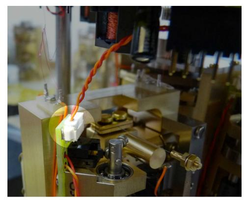
3. Disconnect the cables to the locking motor at the connector shown:
