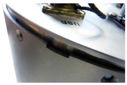
5. Lift the lid away from the cylinder and, wearing an anti-static wrist-band, disconnect (at either end) the ribbon cable connecting it to the lower electronics:
