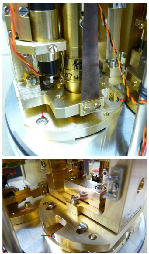
4. Undo the three screws (arrowed in the following photographs) holding the component sensor to the instrument base:
