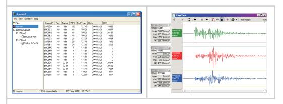
Scream! can **replay archived data** and **convert data** into a number of common formats, including MiniSEED and UFF. Güralp digitizers can also be fully **configured and controlled** using a graphical interface.
