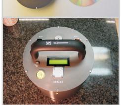
Identical components to the 5T are also used in the CMG-5TB borehole accelerometer. Strong motion borehole instruments can provide important information on the sub-surface soil movements which cause a high proportion of the damage sustained by structures during an earthquake.
