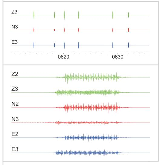
Preliminary results from the station show it working well, recording vibrations on the line resulting from passing trains.
