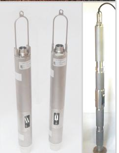
A CMG-5TB module can also be fitted as part of a combined weak- and strong-motion borehole instrument, providing unsurpassed resolution and dynamic range for both local events and teleseisms.
