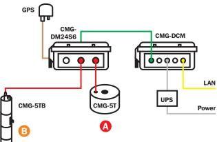
At A and B, on the fault plane, a combined installation includes a CMG-5TB borehole accelerometer at depth, and a CMG-5T instrument in an enclosure on the surface.
