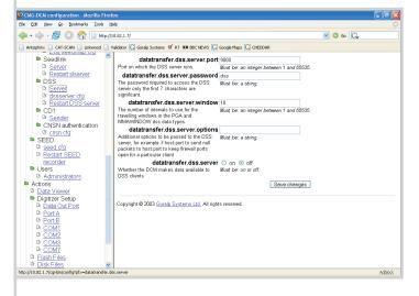
Güralp Systems' DCM data modules also support DSS (Data Subscription Service), a low-latency protocol providing instant access to quantities such as peak and RMS average acceleration levels, spectral intensity, and total horizontal acceleration.
