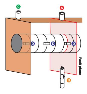
A typical design includes both surface (A) and borehole (B) strong-motion sensors at stations in fault zones along the route of the pipeline.
