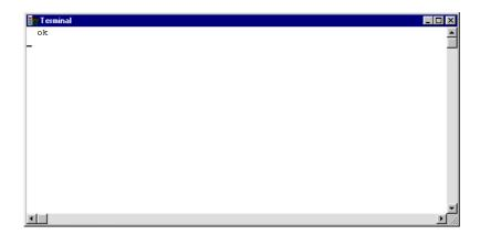
2) If the user presses the **Enter** key "ok" will appear on a new line, signifying that there is two-way communication with the SAM.
