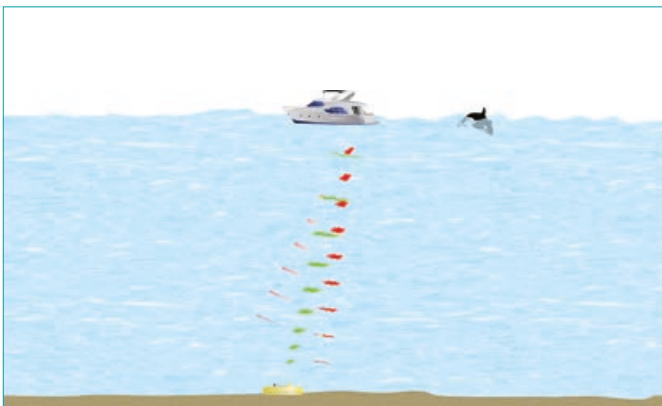
ACOUSTIC TELEMETRY PROVIDES NEAR-REAL-TIME DATA TRANSFER BETWEEN THE AQUARIUS OBS SYSTEM ON THE SEABED AND THE SURFACE
