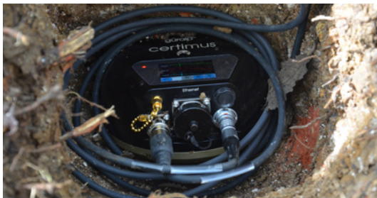
SURFACE BURIAL IS SIMPLIFIED WITH SENSORS THAT ARE FULLY OPERATIONAL AT ±90 DEGREES
