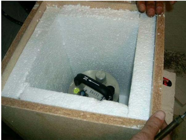
11. Ensure that the sensor cable is loose and that it exits the seismometer enclosure at the base of the instrument. This will prevent vibrations from being inadvertently transmitted along the cable.
