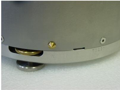
If you cannot easily see the pointers, you should align the sensor using the north arrow on the handle. However, the alignment of the handle with the sensors inside is less accurate than the metal pointers.
