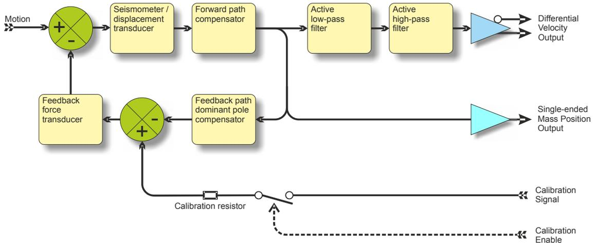
The *hybrid* feedback circuit contains a single capacitor in parallel with a resistor, resulting in a single dominant pole. Below this frequency, which can be varied from the standard 30 seconds, the response of the seismometer is flat to ground acceleration. Above it, the response is flat to velocity. Hybrid-feedback systems provide a stable response, particularly for portable systems, with a high saturation level at high frequencies and a high dynamic range at long periods.
