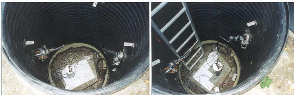
However, noise tests show that this method of installation is significantly inferior to the same concrete plinth with the tiles removed (right). Horizontal sensors show
