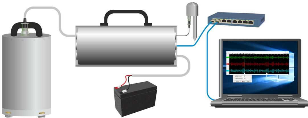
We recommend that you keep the digitiser near the instrument if at all possible, to minimize the length of analogue cable required. Once digitized, the signal is robust to degradation by noise or attenuation. Keeping the digitiser in the quiet, stable conditions of a seismic installation also provides it with an optimum environment for the on-board ADCs.
