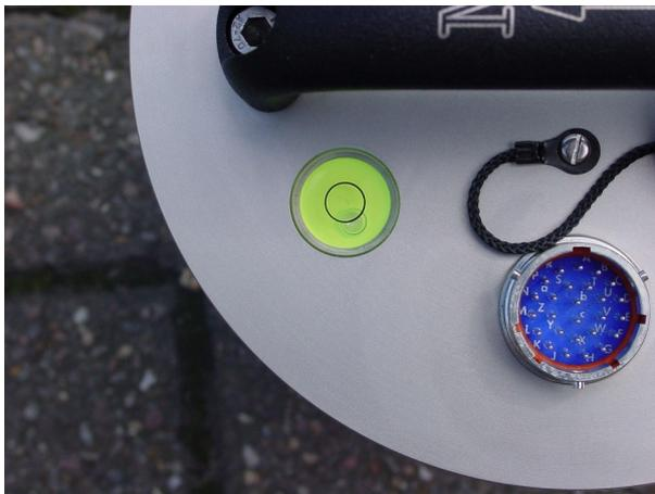
Level the sensor using the adjustable feet of the instrument, until the bubble in the spirit level lies entirely within the inner circle. (The instrument can operate with up to 5° of tilt, but with reduced performance.)
