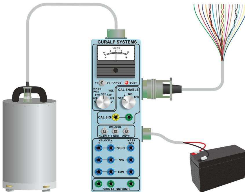
The digitiser can be connected either to the break-out box, as in the previous illustration, or to the hand-held control unit, as shown above.
