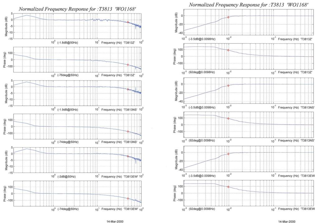
If you want to repeat the calibration to obtain more precise values at a frequency of interest, or to check that a sensor is still functioning correctly, you can inject calibration signals into the system using a Güralp digitiser or your own signal generator, and record the instrument's response.
