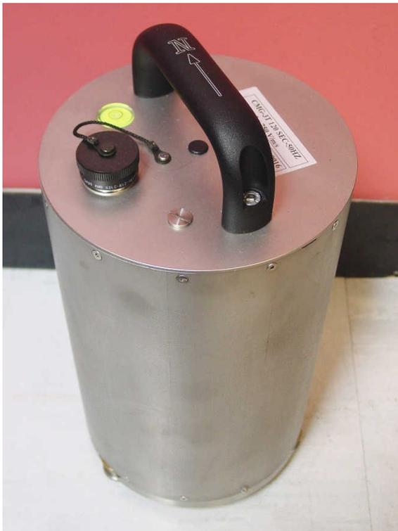
The 3T is designed for mounting on a hard, near-horizontal surface well coupled to the bedrock. After levelling and orienting the case, you can perform accurate adjustments internally by sending the instrument control signals. These electronics allow it to compensate for a tilt of up to 5° from horizontal.
