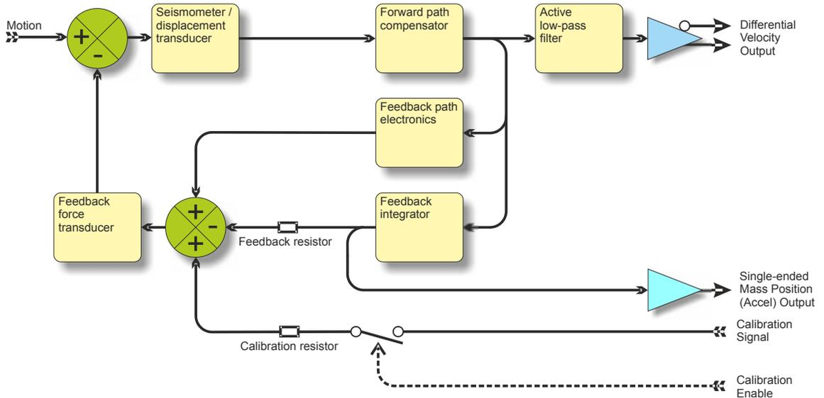
The *conventional-response* feedback system has an additional parallel feedback circuit, consisting of a non-inverting integrator in series with a resistor. This arrangement results in two poles at specified frequencies. The velocity response of a conventional-response system is defined by a transfer function identical to that of a conventional long-period sensor with a damping constant  $\zeta$  of 0.707 ( $1/\sqrt{2}$ )
