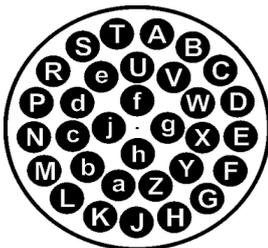
Wiring details for the compatible socket, MEC-GEN-2002-32W, as seen from the cable end (*i.e.* when assembling).
