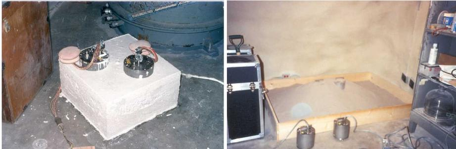
Again, this method produces inferior bonding to the instrument, and moisture becomes trapped between the hard surfaces. We recommend the use of fine dry sand (right) contained in a box if necessary, which can also insulate the instrument against convection currents and temperature changes. Sand has the further advantage of being very easy to install, requiring no preparation.
