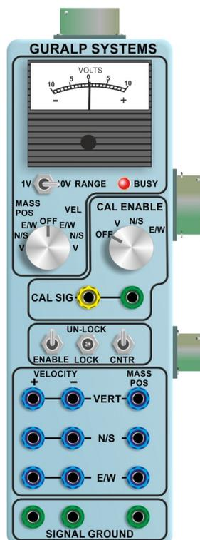
This portable control unit provides easy access to the seismometer's control commands, as well as displaying the output velocity and mass position (*i.e.* acceleration) on an analogue meter. It takes input from the 26-pin connector at the bottom, and repeats it at the connector on the side for connection to further equipment.
