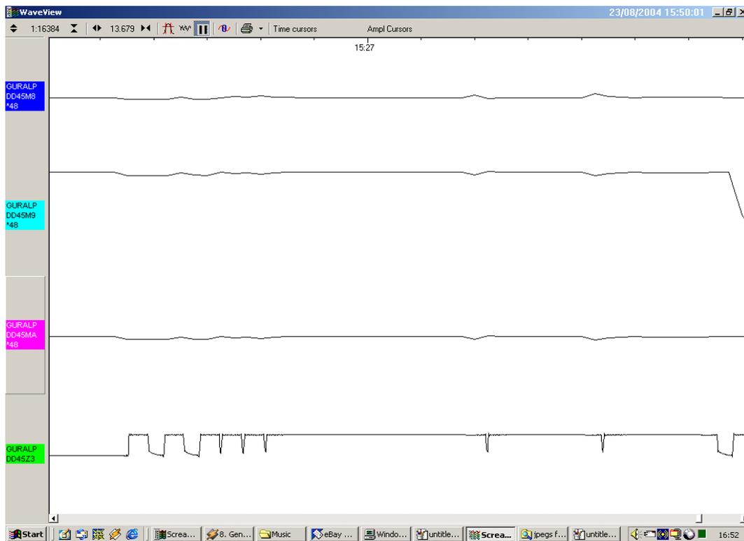
The five-stage process comprises locking the *Z*, *N/S* and *E/W* masses, followed by longer periods tilting the *N/S* and *E/W* sensor base to their end stops. During the latter two periods, the position of the *N/S* and *E/W* masses will “flip” to one side.
