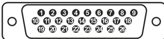
Wiring details for the compatible socket, DA26F, as seen from the cable end, i.e. during assembly
