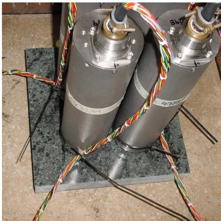
Placing a granite plinth on a sand layer increases the contact between the ground and the plinth and improves the performance of the instrument. There is also no need to mix concrete or to wait for it to set, as in step 5.
