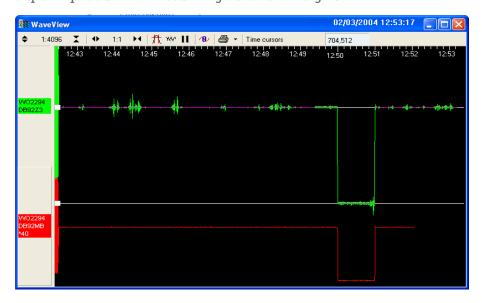
The **Ampl Cursors** button will now be displaying a value, which is the strength of the returning signal in counts (doubled, if using a sine wave). Measure the other two signal strengths in this manner.
