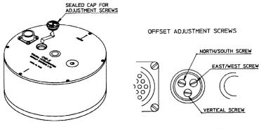
THE OFFSET ADJUSTMENT SCREWS ARE PROTECTED BY A SEALED CAP. UNSCREW AND REMOVE THE CAP TO REVEAL THE ADJUSTMENT SCREWS EACH SCREW ADJUSTS ONE SENSOR, WHICH SERSOR CORESPONDS TO WHICH SCREW IS SHOWN IN THE DETAIL ABOVE ENSURE THAT THE CAP IS REPLACED AND TIGHTENED DOWN FULLY WHEN ADJUSTMENT IS COMPLETE, TO ENSURE PROPER PROTECTION
