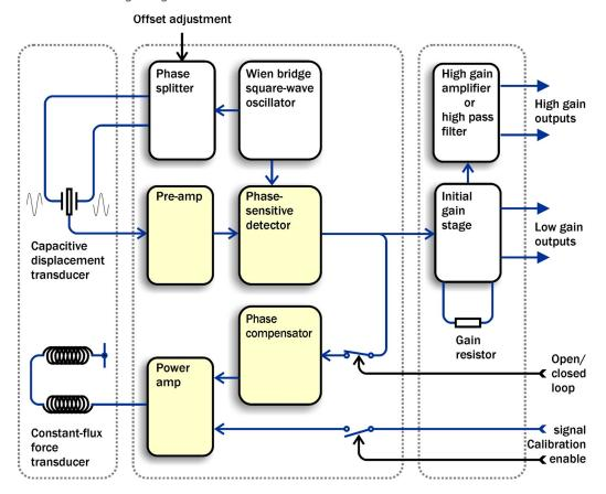
The mass and the capacitor plates are energised by a two-phase transformer driver, forming a differential capacitor. This acts as a capacitive transducer, whose signal is then demodulated with a phase-sensitive detector. The accelerometer feedback loop
