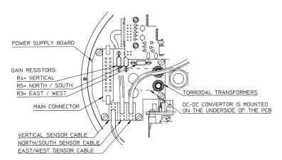
If G is the gain change you require, then the value of the resistors to insert is given by the formula
