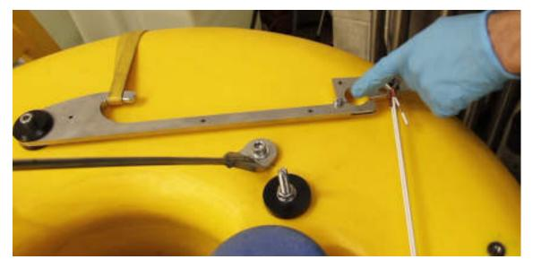
Now pivot the tensioning tool around the inner/smaller notch to bring the two arms together. Take care the ensure that the wire loop passes around the arm and pivot point.
