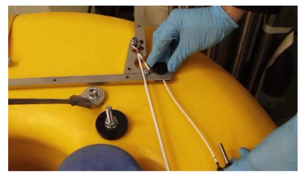
With the burn-wire in place, now release the tensioning tool to transfer the tension of the ballast release system from the tool to the burn-wire itself. Ensure that the tensioning tool wire loop passes cleanly around the burn-wire ends and does not force them from the arm notches.
