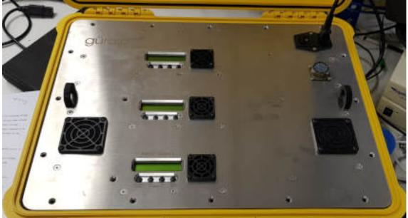
Therefore, three battery chargers were installed in the charger unit, all three are connected to the OBS unit through the same cable described in Section 5.3 on page 23. The charger unit voltage input is 85 V to 230 V AC.
