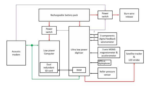
The Aquarius is the sea-floor unit of the system. It includes a weak motion triaxial digital broadband velocity seismometer, which is operational at any angle, without the need of any gimbals system. A three-axis magnetometer and a MEMS accelerometer allow calculation of the main sensor's 3D position on the seabed.
