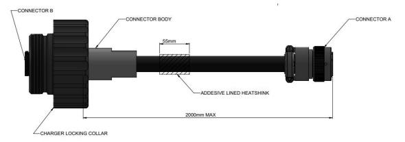
A 2.5 m charging cable, specifically designed for charging the Aquarius has been provided with the system. The cable has a thirty-two-way military-specification bayonet connector on both ends: the socket on the Aquarius canister side and the plug on the charger unit side.
