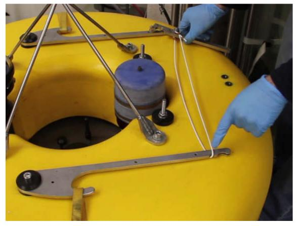
Then align the tip of tensioning tool into the smaller/inner notch in the opposing arm as shown below. Ensure that the retaining washers straddle the arm to prevent the tensioning tool slipping.
