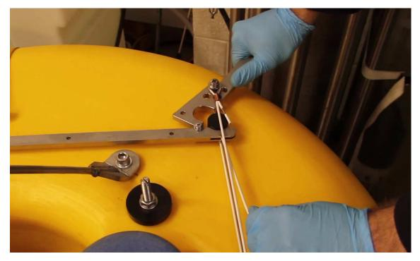
As the tensioning tool is removed, the burn-wire passes completely through the tensioning tool wire loop, including the central potted junction node and cable.
