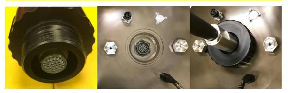
The cable connector with the large black ring connects to the OBS canister. Check the alignment as the connector is pushed in and tightened by hand.
