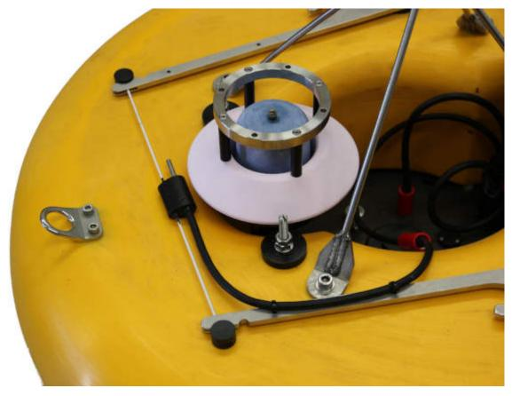
To release the unit a current is passed between the Burn-Wire and a cathode, causing the Burn-Wire to corrode rapidly, thus breaking and releasing the unit. When the Burn-Wire has broken the unit will float to the surface thanks to the lifting force provided by the syntactic foam block.
