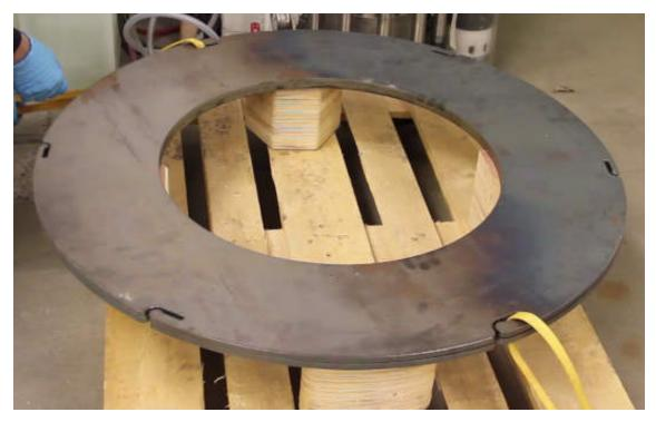
The easiest way to approach this task is to raise the plates off the ground with suitable blocks first, to ensure the lowered Aquarius system sits down on to the ballast plates directly rather than resting on the ground. This can make aligning the circular ridge on the Aquarius buoyancy with the inner circle of the ballast easier, and reduces the force required by the burn-wire tensioning tool (which would otherwise be required to lift the ballast plates before tensioning occurred).
