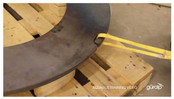
Ensure that the strap loops are located as far into the slots as possible, so they cannot slip out when tension is applied.
