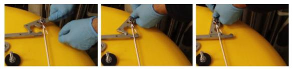
With the arms tensioned with the tensioning tool, insert each end of a new burnwire into the larger/outer notch of each of the arms.
