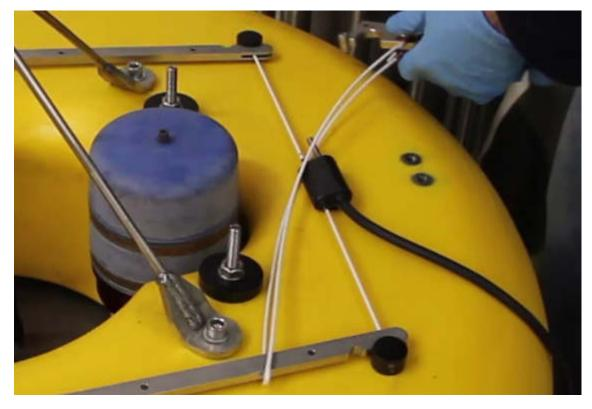
Finally, after cleaning and applying grease as required the two way Subconn burnwire connector may be mated with the cable loom. The electrical operation of the burn-wire should be verified by manually activating the burn-wire from Discovery and assessing the anode to cathode voltage with a multimeter.
