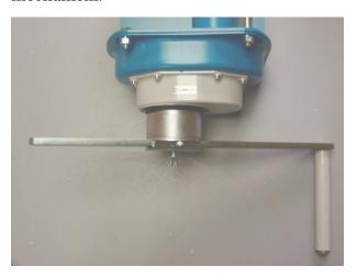
11. Hang the strain relief unit and instrument(s) from the loop at the other end of the cable. You are now ready to lower the assembly into the borehole as described above.
