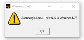
Scream! produces this warning when the reference sensor is not using a standard N/S channel, *i.e.* it is using the auxiliary (X) channel instead. If you are using a separate digitiser, the warning will not appear.
