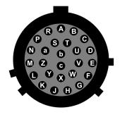
Wiring details for the compatible socket, \*\*\*-16-26S, as seen from the cable end (*i.e.* when assembling).
