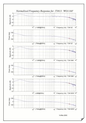
If you want to repeat the calibration to obtain more precise values at a frequency of interest, or to check that a sensor is still functioning correctly, you can inject calibration signals into the system using a Güralp digitizer or your own signal generator, and record the instrument's response.
