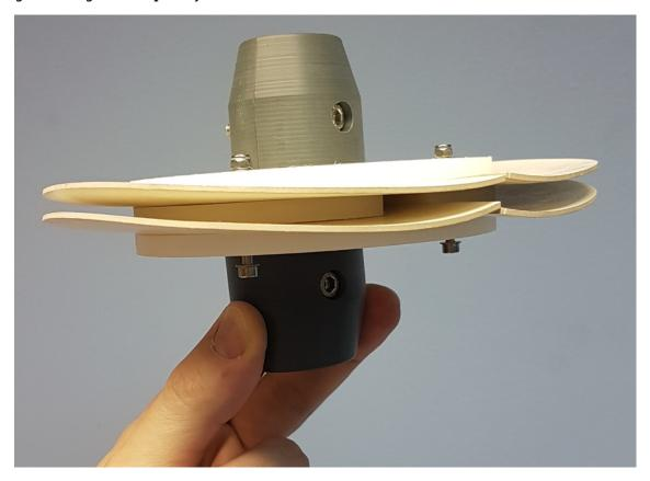
The baffle consists of some large, deformable washers and spacer material attached to a cable clamp. For best results, one should be installed on the signal & suspension cable, half way between the sensor and the surge arrestor. Once in position, it should be tightened onto the cable using the socket-head screws.
