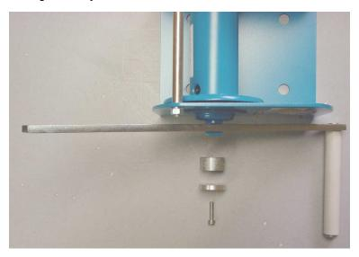
9. Wind the cable onto the winch by rotating the handle. Ensure that the cable builds up neatly across the drum. Continue winding until the loop on the other end is as high as you need it to install the equipment.
