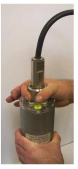
times during tightening in order to ensure that the connector is screwed fully home.
