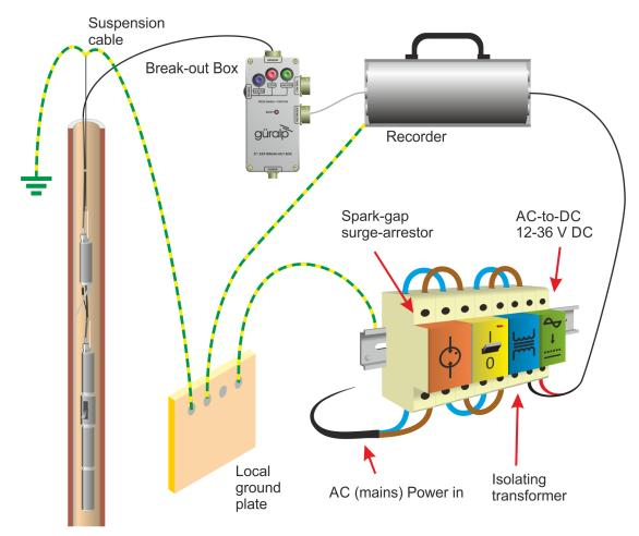
For boreholes with a metallic casing at the bottom and plastic above, we recommend connecting a cable between the sensor housing and the ground plate so that the lower borehole casing acts as the earthing point.
