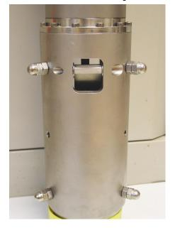
The motor has a power system separate from that of the sensor, and can be controlled from the surface using a hole lock control unit. Once the sonde is installed, the hole lock control unit may be removed. Without power, the hole lock will not be able to retract, and the sensor will be secured.
