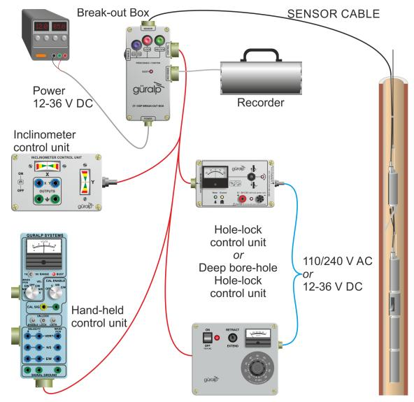
Güralp 3-series instruments are also suitable for installing in boreholes with sand back-fill. In this case no hole lock unit is necessary.
