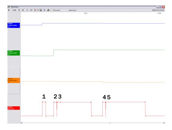
In the five-stage process, each mass in turn is locked with a motorised micrometer (stages 1, 2, 4), and the *N/S* and *E/W* sensor bases are tilted to their end stops (stages 3 and 5). At some point during each tilting stage, the position of the relevant mass will flip to one or other side.
