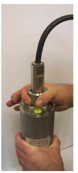
3. If your system does not have a separate surge-suppressor sonde, fix the main lifting cable to the shackle on top of the strain relief mechanism and run the signal cable through the mechanism using the built-in clamps (without tightening them). Otherwise, fix the main lifting cable to the shackle on top of the surge-suppressor sonde.
