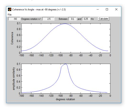
The two-stage algorithm rotates the N/S and E/W components of the sensor being tested in small steps. It measures first the amplitude similarity, and then the coherence between the virtual (rotated) N/S component and the reference N/S component, for a number of rotation angles.
