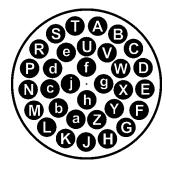
Wiring details for the compatible socket, MEC-GEN-2002-32W, as seen from the cable end (*i.e.* when assembling).
