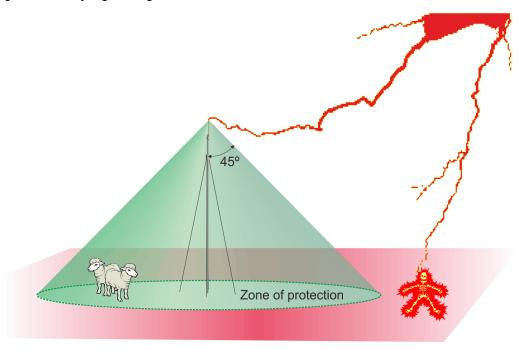
These should lead to grounding point well away from the borehole. As a rule of thumb, a lightning mast provides a "zone of protection" within a 45° cone descending from the top of the mast.
