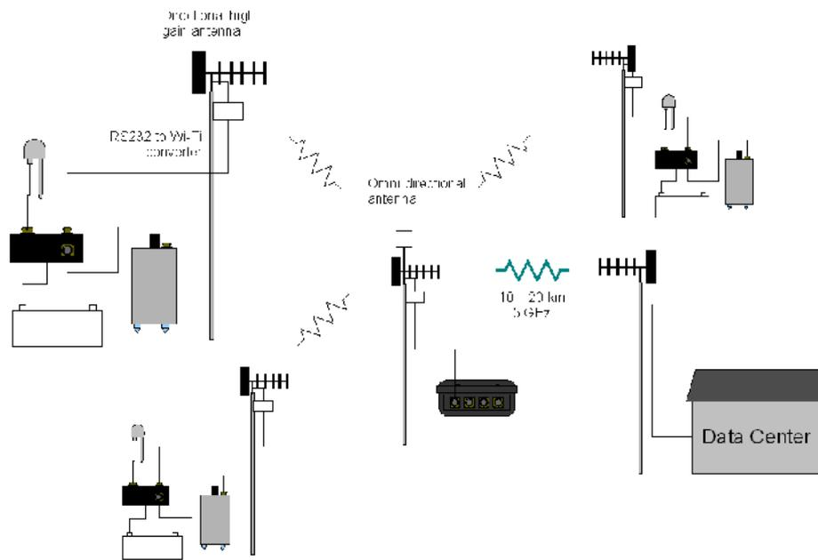
At this location, which can be up to 500 metres away, a low-power CMG-EAM data module might act as an access point for the array elements and forward data onto a higher-bandwidth radio link.
