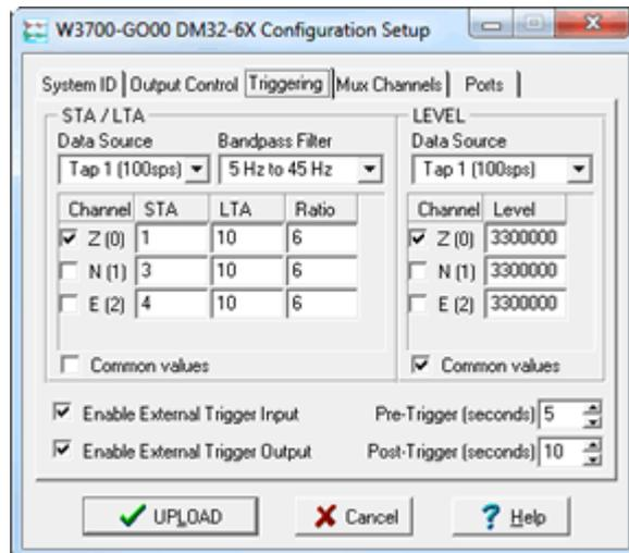
The CD24 can be set up for triggered output, that is, to output certain data streams only when a particular trigger criterion is met. The trigger criterion can be tested with data from the same or some other stream. For example, you could use a later tap (with a lower sample rate) as a trigger for output from an earlier, more detailed tap. Scream! 4 (and above) also allows you to configure each digitiser to receive triggers from other digitisers.
