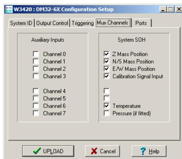
If a tick is placed in the box next to a channel, its data will be collected and transmitted as a data stream in GCF format, just as with the normal data channels. To indicate that the data come from a Mux
