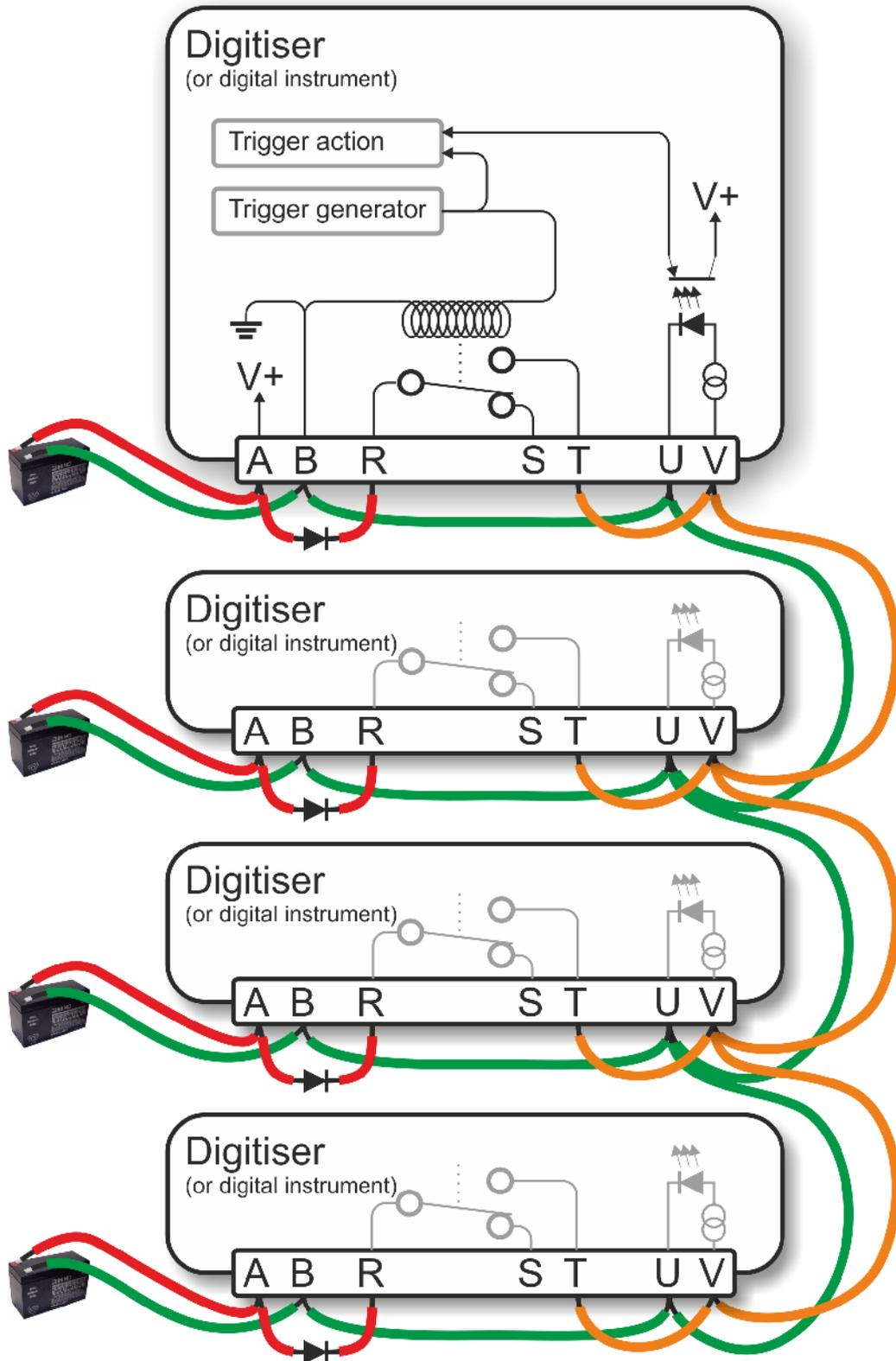
The diode between pins A and R is important, because if two digitisers generate a trigger simultaneously, their power supplies will both be connected via the internal relay contacts to the common trigger line on pins V, and hence connected together. This can cause considerable current flow with consequent risk of fire, as well as severe damage to equipment and cables.
