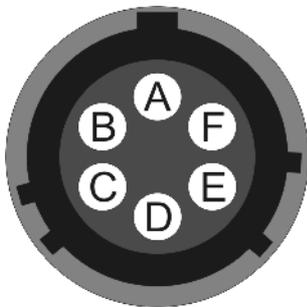
Wiring details for the compatible plug, \*\*\*-10-06P, as seen from the cable end (*i.e.* when assembling).
