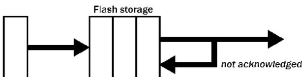
Instructs the CD24 to begin writing blocks to Flash memory as for *FILING* mode, but also to transmit data to clients. Data are transmitted in strict order, oldest first; the CD24 will only transmit the next block when it receives an explicit acknowledgement of the previous block.
