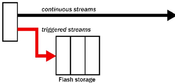
Instructs the CD24 to transmit continuous streams directly to clients as for *DUPLICATE* mode, but to store triggered data *only* into Flash storage.
