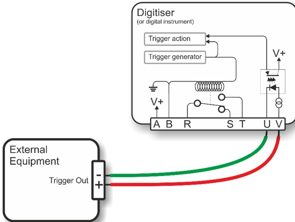
To trigger a digitiser from an external source which provides a triggering voltage, you merely need to connect the external trigger voltage to pins U and V of the digitiser as shown above. The voltage can be anywhere between 4 and 40 V DC as the constant current circuit protects the LED of the optoisolator.
