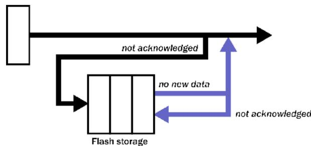
Instructs the CD24 to transmit current blocks to clients if possible, but to store all unacknowledged blocks in the Flash memory and re-send them, oldest first, when time allows. *ADAPTIVE* mode is best suited for “real-time” installations where the link between digitiser and client is intermittent or difficult of access.
