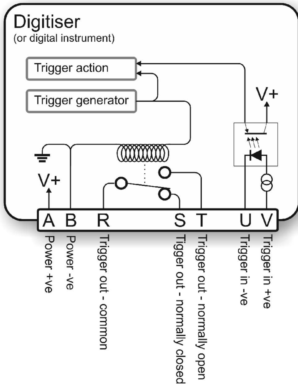
The *Trigger Out* relay is *not* activated if you provide a *Trigger In* voltage. The digitiser must trigger *itself* for the relay to switch. This arrangement prevents any trigger loops from occurring.
