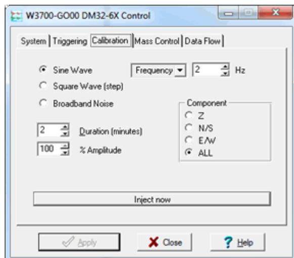
Each channel calibrates the corresponding component of the instrument. Select one or all components for calibration.
