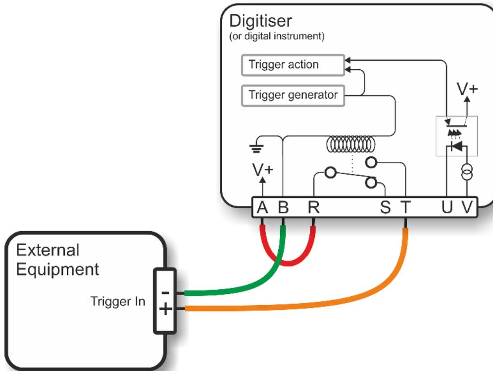
If your equipment can trigger from the same voltage as the CD24's power supply, the simplest arrangement is to use the voltage across the sensor's power supply as the trigger supply.
