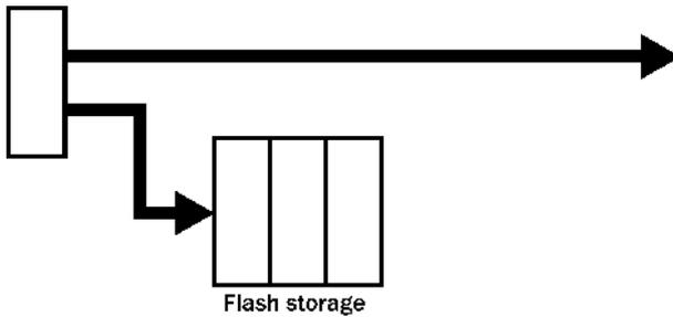
Instructs the CD24 to transmit streams directly to clients as well as storing all data into Flash storage as for *FILING* mode.
