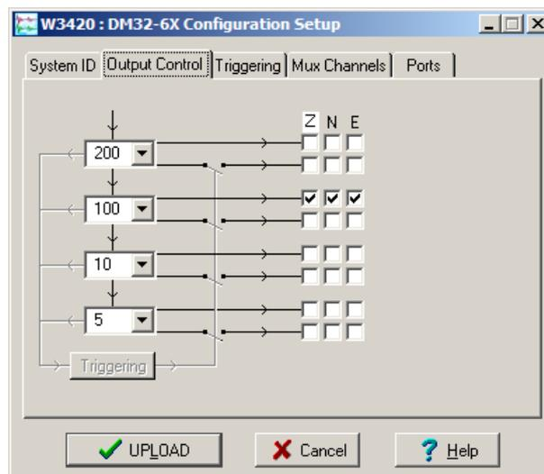
The CD24 initially samples incoming data at 2000 Hz. These data are then filtered and reduced to a lower rate (*decimated*) using an on-board digital signal processing unit, or DSP. The DSP has several filtering-decimation stages, which run one after the other. Stages which can produce output (and the outputs from those stages) are called *taps*. The CD24 can output 4 taps simultaneously.
