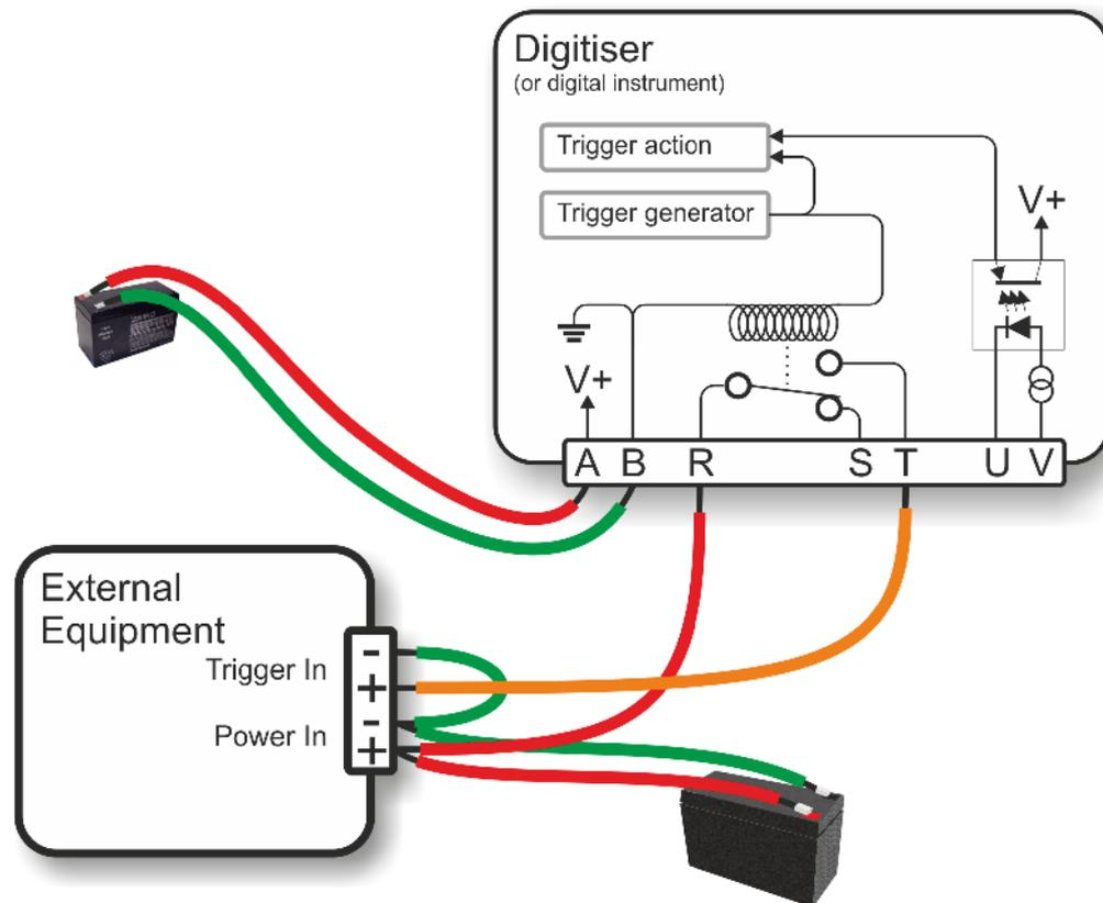
The diagram above illustrates how to trigger the external equipment using its own power supply, which is connected to the trigger input via the normally-open relay contacts (pins R and T).
