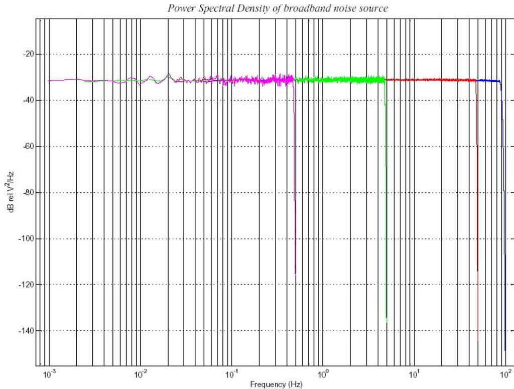
The different coloured lines show the results of experiments which measure the power spectral density over several frequency bands. Together, the results show a flat noise level over the entire passband to within experimental error.
