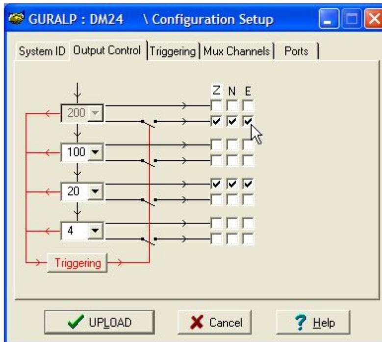
To the right of each decimation factor menu is a grid of check-boxes. These boxes mark which streams of data to generate at each sample rate. The screen-shot above shows a possible configuration for a triaxial instrument. Every channel of the digitiser may be output at any tap; currently, all three axes are being output at Tap 2 (20Hz).
