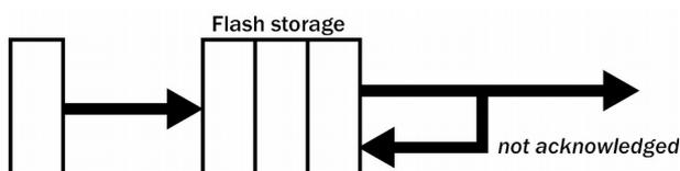
Instructs the digitiser to begin writing blocks to Flash memory as for FILING mode, but also to transmit data to clients. Data are transmitted in strict order, oldest first; the digitiser will only transmit the next block when it receives an explicit acknowledgement of the previous block. If the communications link is only marginally faster than the data rate, it will take some time to catch up with the real-time data after an outage.
