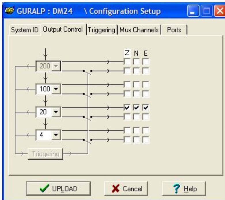
Güralp digitisers initially sample incoming data at a high rate (e.g. 512,000 Hz for the DM24), which is then filtered and reduced to a lower rate (decimated) using an on-board digital signal processing unit, or DSP. The DSP has several filtering-decimation stages, which run one after the other. Stages which can produce output are called taps. The Güralp DM24 can output 4 taps simultaneously. The input to the tap chain is fixed at 2,000 samples per second.
