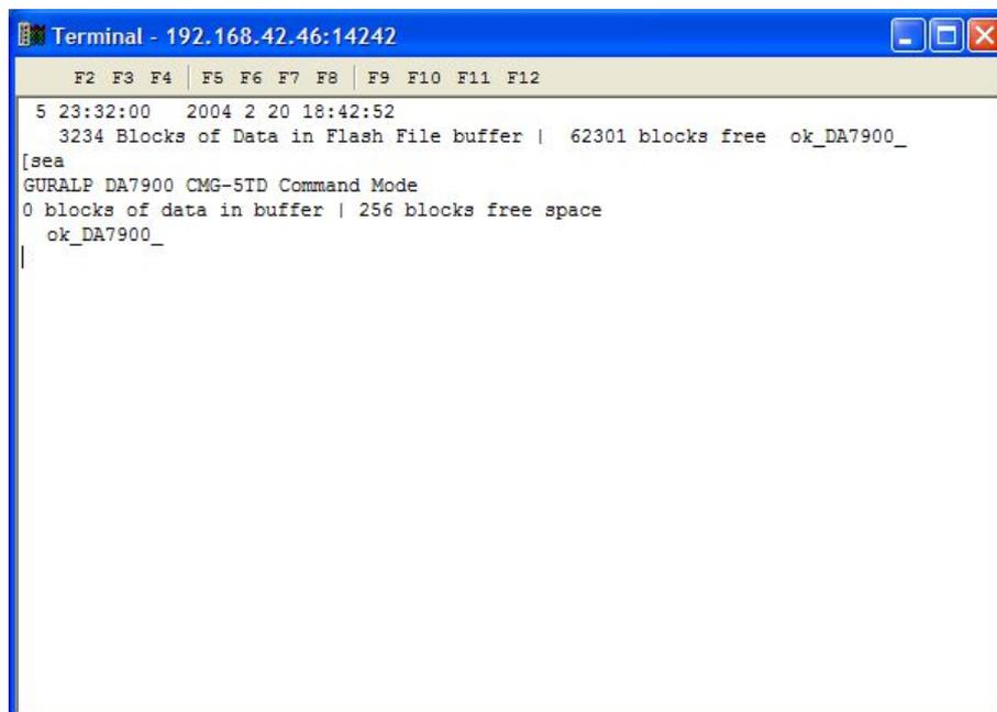
Check that there is two-way communication with the digitiser by pressing Enter. The digitiser should reply with `ok` on a new line. Type `re-boot` to reinitialize the digitiser, and confirm with `y`. As it is restarting, the digitiser will report its status over the terminal connection, followed by a maintenance menu:
