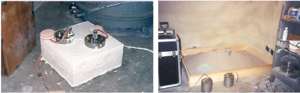
Again, this method produces inferior bonding to the instrument, and moisture becomes trapped between the hard surfaces. We recommend the use of fine dry sand (right) contained in a box if necessary, which can also insulate the instrument against convection currents and temperature changes. Sand has the further advantage of being very easy to install, requiring no preparation.
