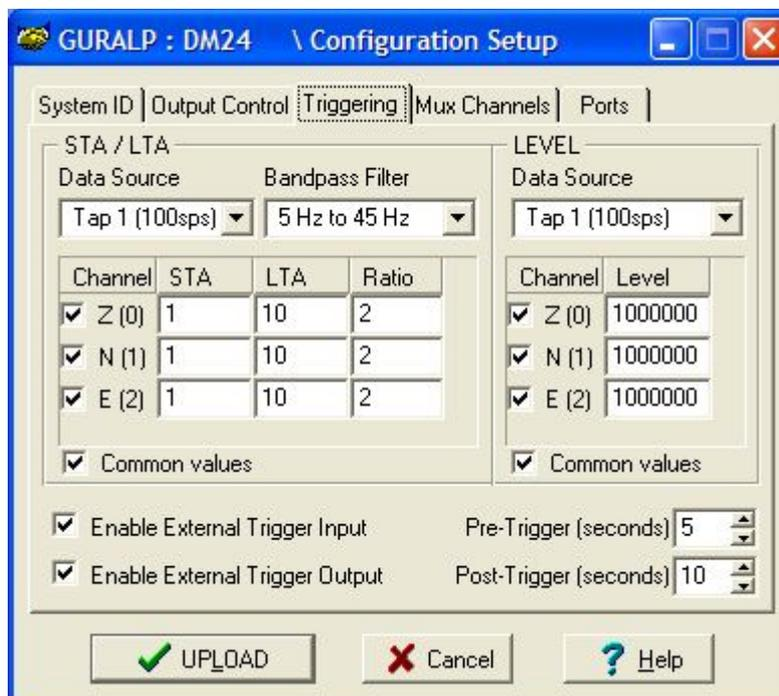
There are two triggering algorithms which Güralp digitisers can use: STA/LTA and level-triggering. In addition, software and external triggering options are available.
