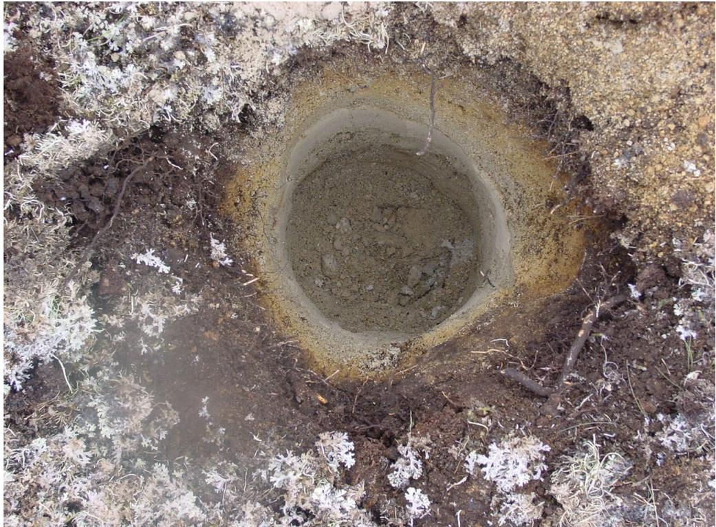
3. If the bottom of the hole is made of hard rock, you may need to put in some loose sand or soil so that the sensor can be levelled.
