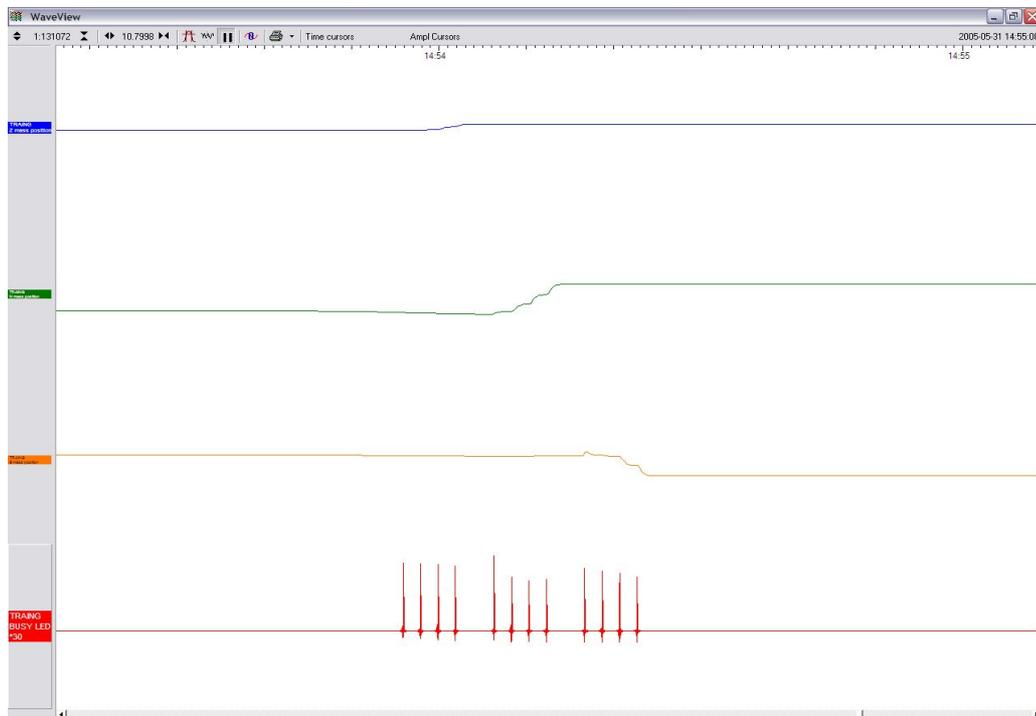
1. The `BUSY LED` pulses to indicate that it is centring the Z component. Each pulse corresponds to a small force on the mass. The pulses become briefer as this goes on, until a pulse is missed, signifying that no corrective impulse is needed.
