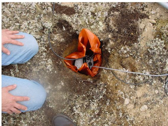
6. Press the sensor down firmly into the soil, without tapping or hitting it.
