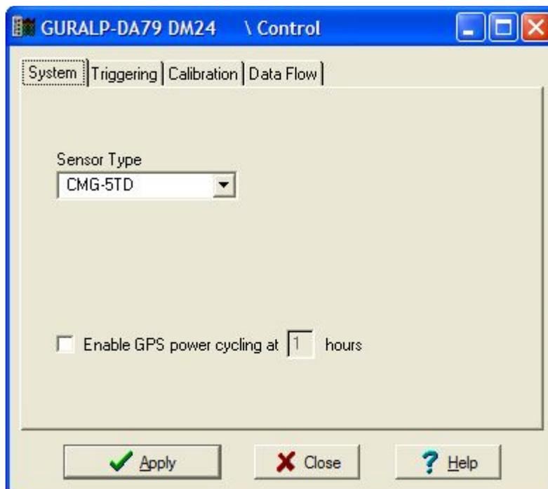
**Sensor Type:** If the sensor attached to the digitiser is a Guralp velocity sensor, you can send control commands to it from the Mass Control tab (see below). Which functions are available on this tab depends on the Sensor Type you have set here. The correct value for your 3ESPCD is "CMG-3T / ESPC"
