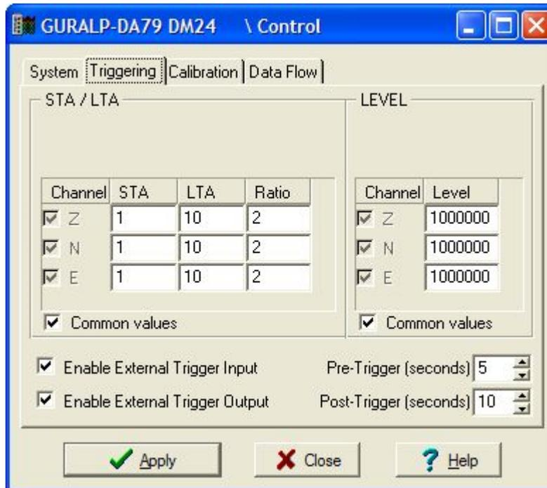
The Triggering pane is very similar to the corresponding pane of the Configuration set-up window although not all options are available, since some require rebooting the digitiser. See “Triggering” in section 5.2.2 on page 53 for more details.
