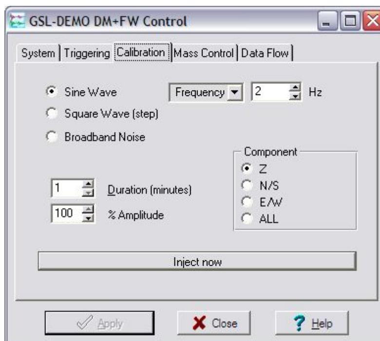
2. Select the calibration channel corresponding to the instrument, and choose Broadband Noise. Select the component you wish to calibrate, together with a suitable duration and amplitude, and click Inject now. A new data stream, ending Cn (n = 0 - 7) or MB, will appear in Scream!'s main window containing the returned calibration signal.
