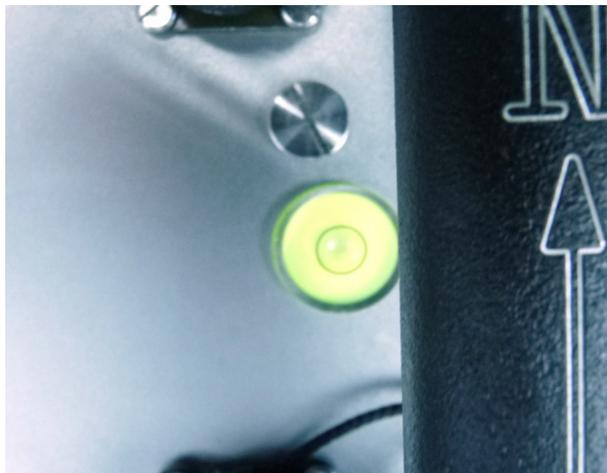
Level the sensor using each of the adjustable feet of the instrument in turn, until the bubble in the spirit level lies entirely within the inner circle. (The instrument can operate with up to 2° of tilt, but with reduced performance.)
