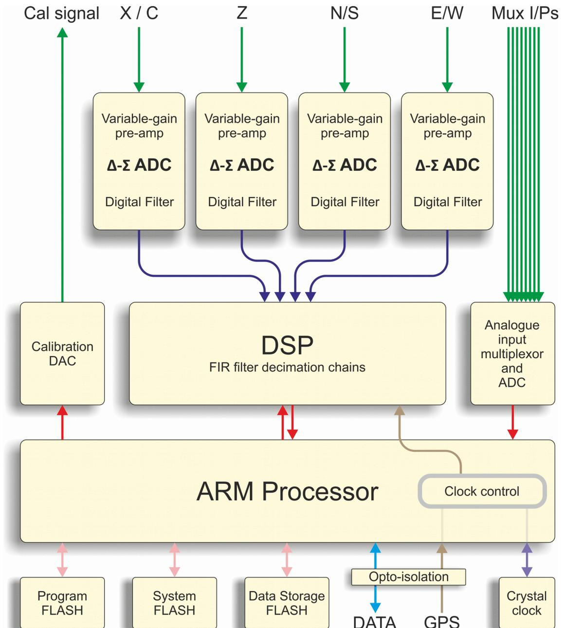
The system is designed around a low power, high performance ARM microprocessor. This is a 32-bit processor with a large address space for data storage and manipulation. It also includes many integrated functions such as multiple timers and serial I/O ports. In addition, the system contains a Cirrus Logic CS5376 digital filtering chip-set and TMS320VC33 digital signal processor
