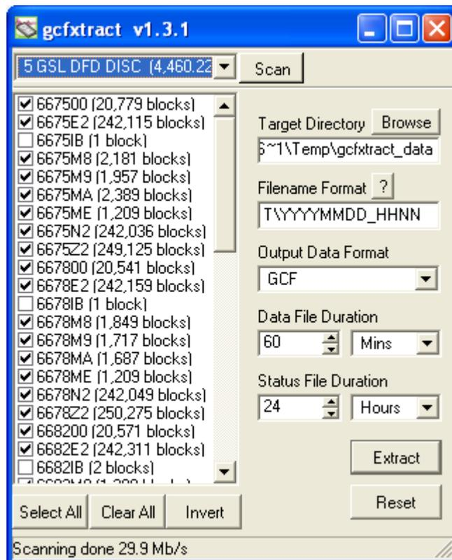
The program will first search for non-DOS disks on all the interfaces it understands. If it does not find your disk, check that it is properly connected and that any relevant drivers have been installed, then click the **Scan** button.
