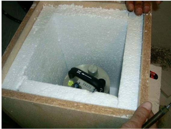
11. Ensure that the cables are loose and that they exit the seismometer enclosure at the base of the instrument. This will prevent vibrations from being inadvertently transmitted along the cables.
