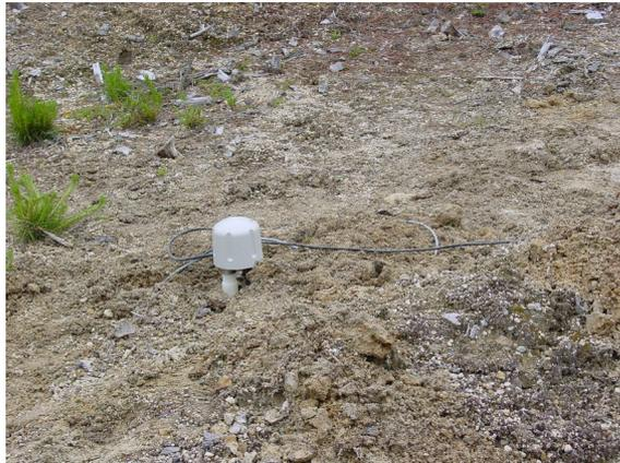
17. If possible, place the GPS near the instrument so that it can be found more easily, and the connector package near the GPS so you can retrieve data from the instrument without affecting the installation.
