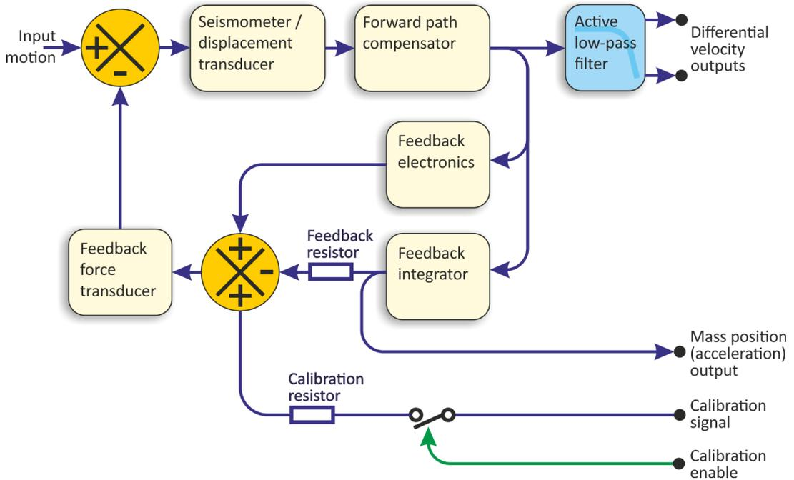
This arrangement results in two poles at specified frequencies. The velocity response of a conventional-response system is defined by a transfer function identical to that of a conventional long-period sensor with a damping constant  $\zeta$  of 0.707 ( $1/\sqrt{2}$ ).
