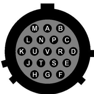
Wiring details for the compatible socket, \*\*\*-14-19S, as seen from the cable end (*i.e.* when assembling).
