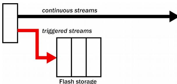
Instructs the digitiser to transmit any continuous streams directly to clients as for DIRECT mode, but to store triggered data into Flash storage as for FILING mode. If you choose DUAL mode but do not select any continuous streams for output, the instrument will send heartbeat messages as for FILING mode. Scream! can pick these up and download new data as necessary.
