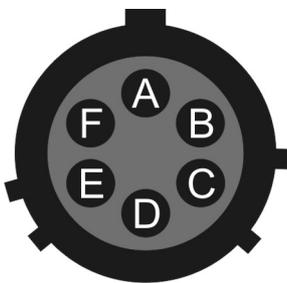
Wiring details for the compatible socket, \*\*\*-10-06S, as seen from the cable end (*i.e.* when assembling).
