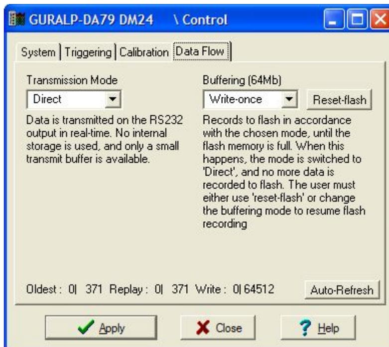
Clicking Apply in this window immediately activates the transmission mode you have selected—there is no need to reboot. If you prefer, you can use the digitiser terminal to switch between transmission modes. The commands to use, which take effect immediately, are given below.
