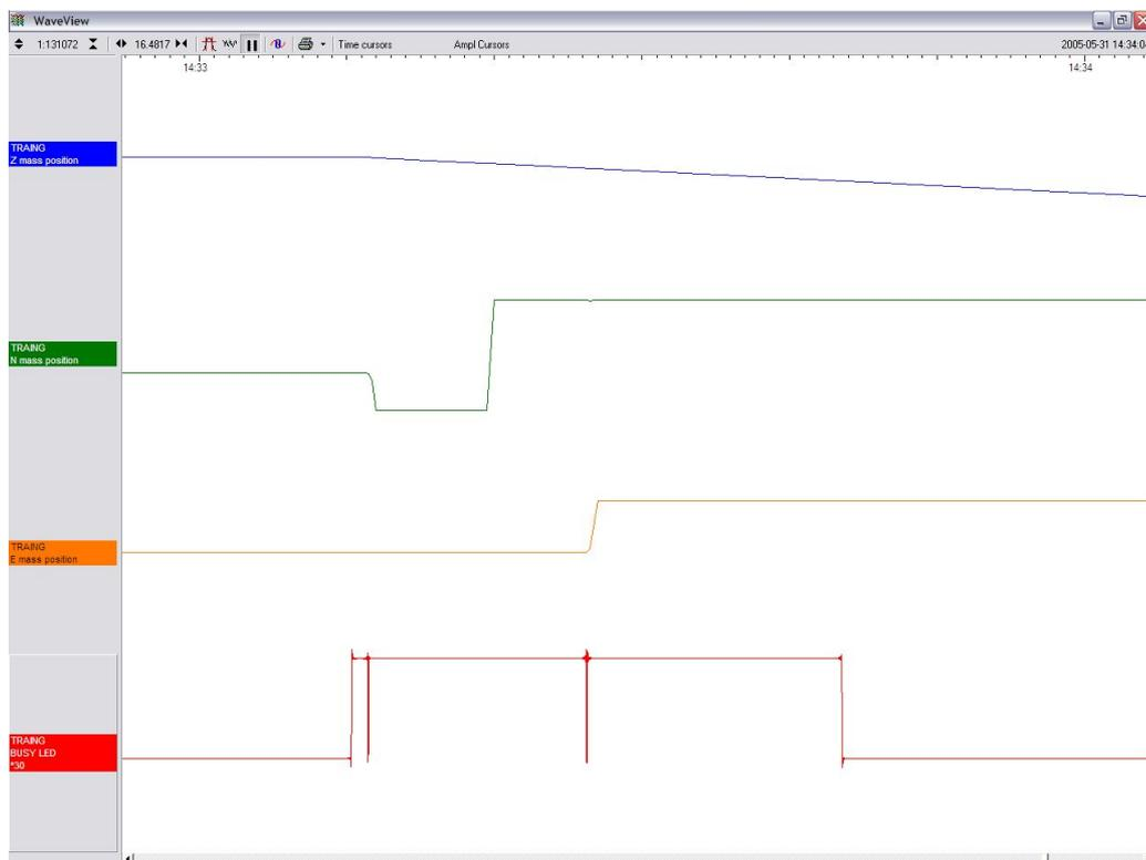
In the three-stage process, the vertical mass is locked with a motorised micrometer, and the N/S and E/W sensor bases are tilted to their end stops. At some point during each tilting stage, the position of the relevant mass will flip to one or other side. With the horizontal bases tilted, gravity will keep the masses pressed against their end stops, effectively locking them in place.
