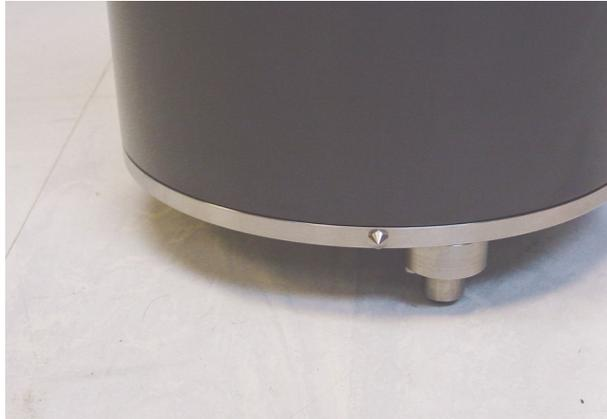
If you cannot easily see the pointers, you should align the sensor using the north arrow on the handle. However, the alignment of the handle with the sensors inside is less accurate than the metal pointers, so they should be used wherever possible.
