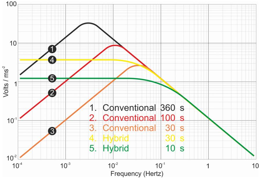
The graph above shows the response in terms of output against input acceleration in units of V/ms<sup>-2</sup>, whilst the second graph is plotted in terms of output against input velocity, in V/ms<sup>-1</sup>.
