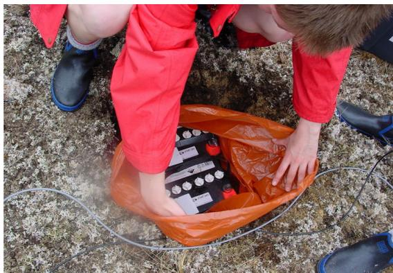
20. Tie the bag and fold over, to make the battery as waterproof as possible.
