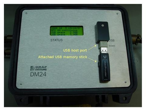
This interface enables the DM24 to record GCF data to a standard USB disk drive or Flash memory stick using the ISO 9293 FAT filing format – readable by Linux, DOS, Windows and Mac OS.
