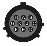
Wiring details for the compatible socket, \*\*\*-12-10S, as seen from the cable end.
