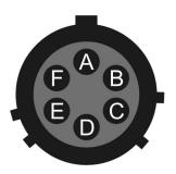
Wiring details for the compatible socket, \*\*\*-10-06S, as seen from the cable end.
