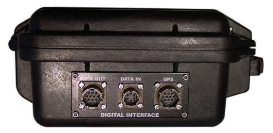
The DM24 transmits data through its DATA OUT port. This is an RS232-compatible serial link, outputting data in GCF format according to the particular configuration of the instrument. The DM24 has a default baud rate of 38,400. You can change this from the command line using the BAUD command or from Güralp Systems' control, acquisition and monitoring software package, Scream! (see Chapter 5 on page 35).
