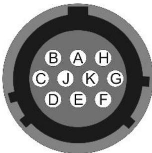
Wiring details for the compatible plug, \*\*\*-12-10P, as seen from the cable end (i.e. during assembly).
