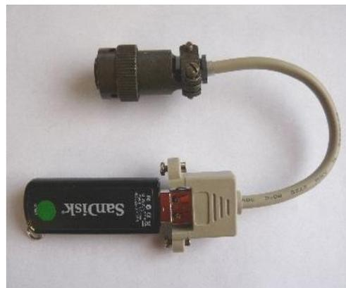
The adapter cable is required when upgrading the firmware of a CMG-DCM, a CMG-EAM and most CMG-DAS units but not when upgrading a CMG-NAM.
