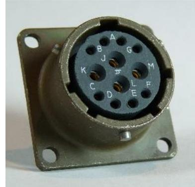
The USB lines provide external host access to the internal USB memory device. When power is sensed on pin J, an internal switch disconnects the memory device from the internal circuitry and connects it to this socket.
