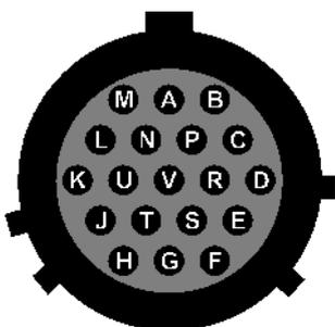
Wiring details for the compatible socket, \*\*\*-14-19S, as seen from the cable end (i.e. during assembly).
