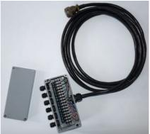
Each of the four breakout boxes has terminal connectors for up to 6 channels and connects to the DAS using 32 pin mil spec connectors.
