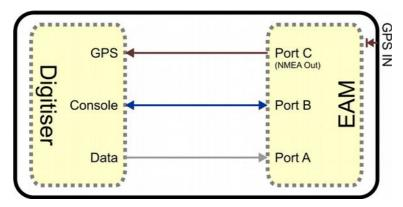
Both the digitiser's GPS input and Port C of the acquisition module must run at 4,800 Baud. This should never be changed. Note that, in this mode, the external GPS socket is disconnected: it cannot be used as an output for additional digitisers.
