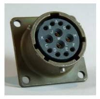
The USB lines provide external host access to the internal USB memory device. When power is sensed on pin J, an internal switch disconnects the memory device from the internal circuitry and connects it to this socket.
