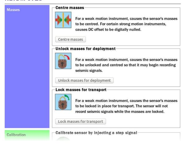
The first part of the screen offers controls to centre, unlock and lock the instrument's masses.
