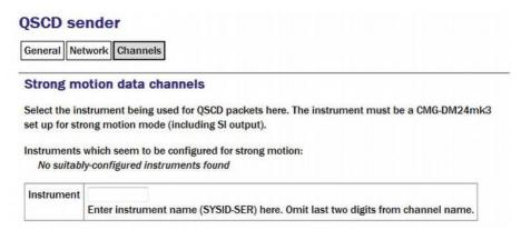
**Instrument:** The acquisition module scans all incoming data and prepares a list, in the correct format, of the names of instruments which are sending strong motion results. Enter one of these names in the field.
