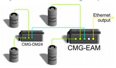
If the output link is over a network, all external serial ports of a standard CMG-EAM (including the "DATA OUT" port) are available for connection to digitisers or digital instruments, allowing up to eighteen channels to be aggregated. An arbitrary number of CMG-EAMs may be chained together, allowing for even more extensive arrangements.
