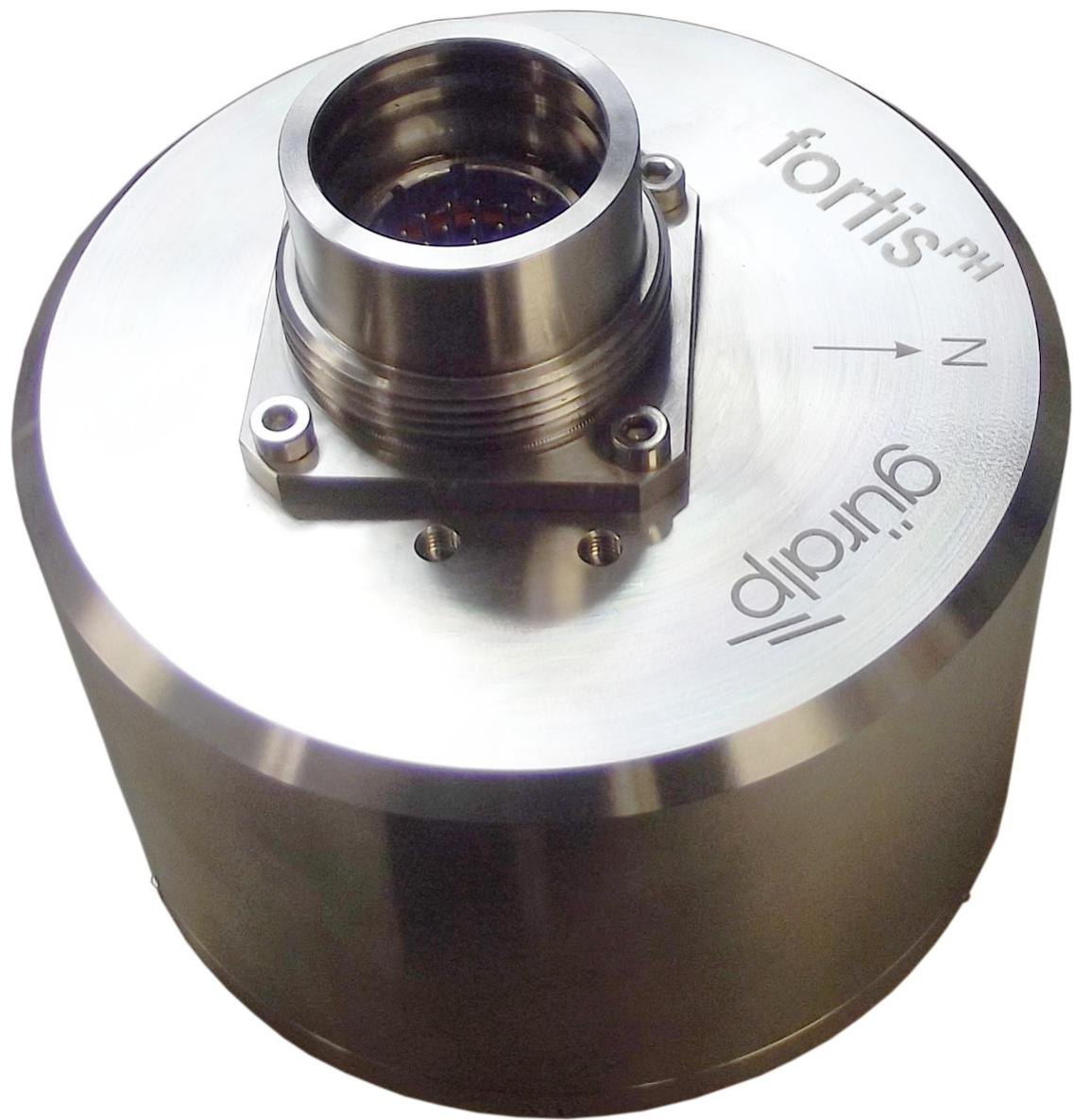
The Fortis accelerometer is also available in borehole-specific packaging. This variant is called the Fortis Post-hole, or Fortis<sup>PH</sup>. The components and electronics inside the sensor are identical to the surface module: the only difference is in the external casing and the connector, which is water-proof to 100 Bar (equivalent to 10 MPa or 1500 psi). See section 7.2 on page 33 for pin-out details.
