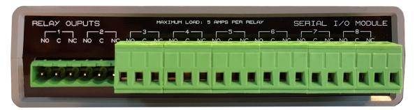
The terminal block can be removed from the I/O Expander Module by pulling directly outwards with moderate force. In the illustration above, the first two blocks have been removed.
