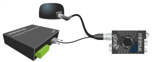
If no analogue sensor connection is required, a simple point-to-point (non-'Y') cable, part number CAS-MIN-0006, should be used:
