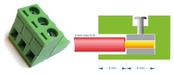
Insert the prepared wire fully into the contact block and fully tighten the screw using a 3 mm flat-headed screw-driver. Check that no loose strands protrude.
