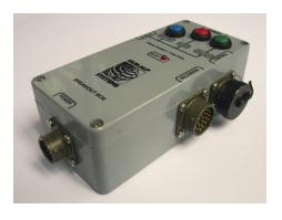
If you are using a breakout box, connect the signal cable between the sensor and the SENSOR connector of the breakout box, and connect the POWER connector to your power supply.
