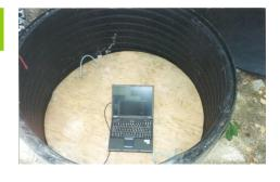
If you are installing in a cased pit (as in this picture), install the digitizer and power supply inside if possible, then seal the installation with a weatherproof cover.
