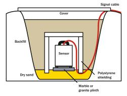
Check you have all necessary equipment and select a suitable location for the pit installation. You will need:
