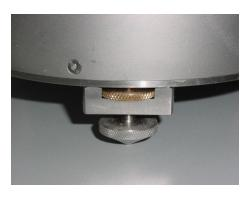
Loosen the brass locking nut on one of the adjustable feet, then turn the foot, screwing it in or out to level the sensor. Check using the spirit level on the sensor lid.
