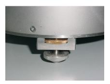
Loosen the brass locking nut on one of the adjustable feet. Turn the foot, screwing it in or out to level the sensor. Check using the spirit level on the sensor lid.
