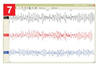
Select some data streams and double-click. A *Waveview* window will open on the streams. Check that the output responds to vibrations near the sensor.
