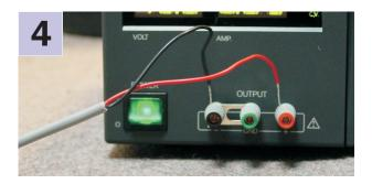
Switch on the power supply and measure the current through the instrument. With the GPS connected and running, the current should be around 120 mA. Once a fix has been obtained, the digitizer will power down the GPS, and the current will drop to around 90 mA.
