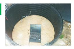
If you are installing in a cased pit (as in this picture), install the digitizer and power supply inside if possible, and seal the installation with a weatherproof cover.
