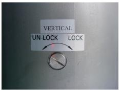
Remove the screw cap protecting the vertical lock access socket, and insert an Allen key. Find the retaining screw within, and loosen it to unlock the vertical component. Repeat for the north/south and east/west components.
