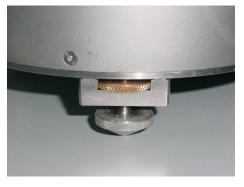
Loosen the brass locking nut on one of the adjustable feet.
