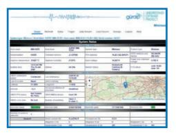
Launch Discovery software. The serial number (as shown on the base of the Minimus) should appear in the main window. If the instrument does not appear, check your Ethernet connection and then press the **Scan Locally** button (more troubleshooting details in Minimus user's manual in section 4.1). Right-click the instrument and select **Live View** then **GDI**.
