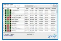
The Live View window will open and start streaming all available data from the Radian. Streams can be added or removed from the viewer using the **Channel List** panel on the left-hand side. Amplitude and time zoom/pan can be controlled using the keyboard arrow-keys or the mouse-wheel.
