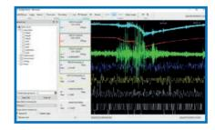
To configure the Radian system (view instrument state-of-health information, configure station metadata and network preferences, manage data storage and data flow), right-click on the Minimus in Discovery's main window and select **View Web Page**.
