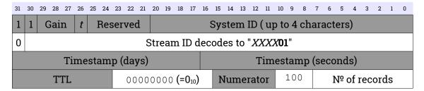
A Unified Status block is a binary, machine-readable block of status information that is emitted every second by a digitiser (when this mode is enabled). The length of the
