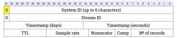
There is no information in the first word other than the System ID itself. Decoding the base 36 IDs is explained in section 2.3 on page 5. The type of digitiser that
