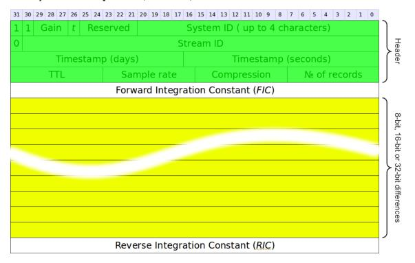
The largest permitted GCF packet contains 250 records. This can hold up to 250, 500 or 1000 sample differences, depending on the Compression code. Together with the four-word header and a word each for the FIC and RIC, the total packet is 256 words, or 1 kB long.
