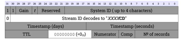
This format is deprecated. Use unified status instead. When CD status packets are enabled, the digitiser will emit one such packet each second.
