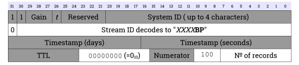
Some digitisers have a 'byte pipe' mode, used to package arbitrary binary data read from an auxiliary serial port into a GCF packet for transmission to a host. The length of the packaged data, in bytes, is given by multiplying the unsigned 8-bit value of the  $N^{\circ}$  of records field by 4. The data are transmitted raw, with no encoding.
