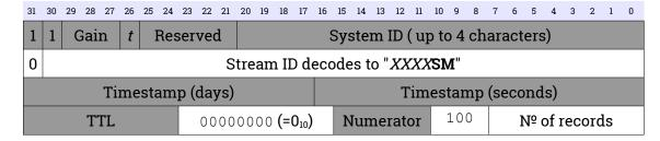
A Strong Motion packet contains the results of strong motion calculations, computed every second by a digitiser (if this mode is enabled). The length of the data, in bytes, is determined by multiplying the unsigned 8-bit value of the  $N^0$  of records field by 4.
