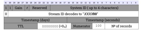
A status block contains textual information such as state of health in ASCII (although there are various control codes and other unprintable characters that may occur, so the data must be sanitised before displaying on a terminal etc.).
