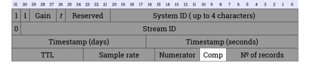
• Code 4 is used to store up to 1000 difference values in 8-bit fields, four per record. Each value must be between -128 and +127 inclusive.
