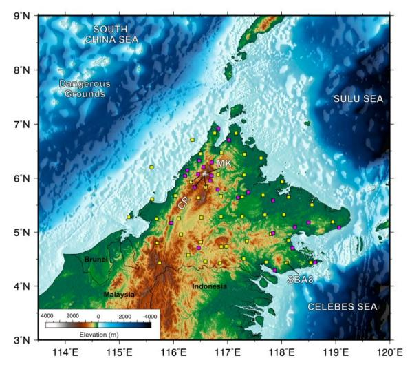
*Figure 2: the nBOSS temporary seismic stations (yellow squares) were deployed with an average station separation of 32km. Pink squares represent the permanent stations operated by MetMalaysia. Image courtesy of Pilia et al., (2023)*
