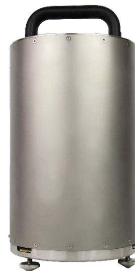
Figure 2. Example of a Güralp '3T' seismometer.
