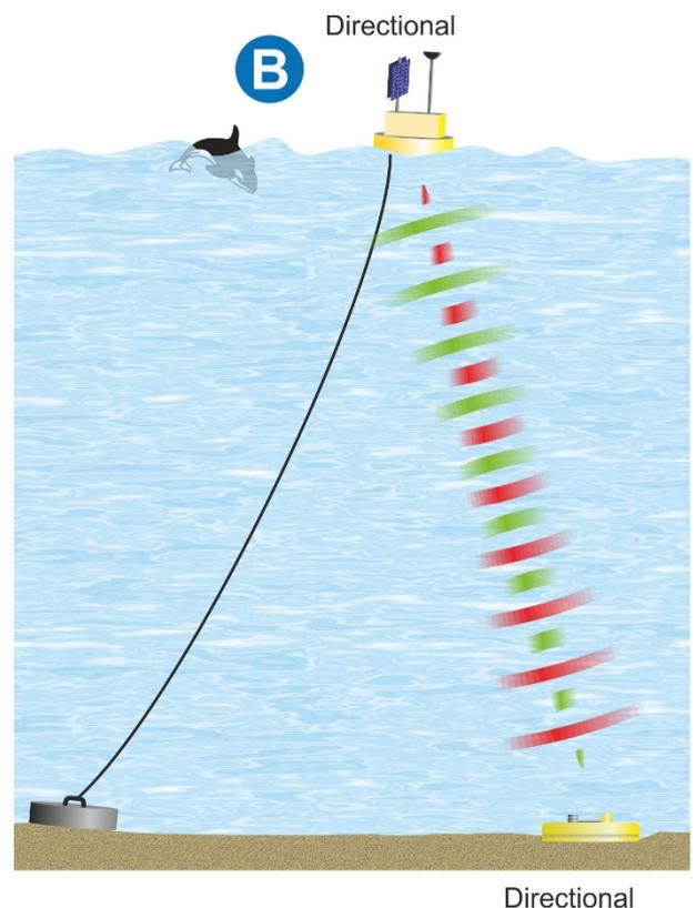
Figure 3 Directional transducers, ocean bottom and topside.
