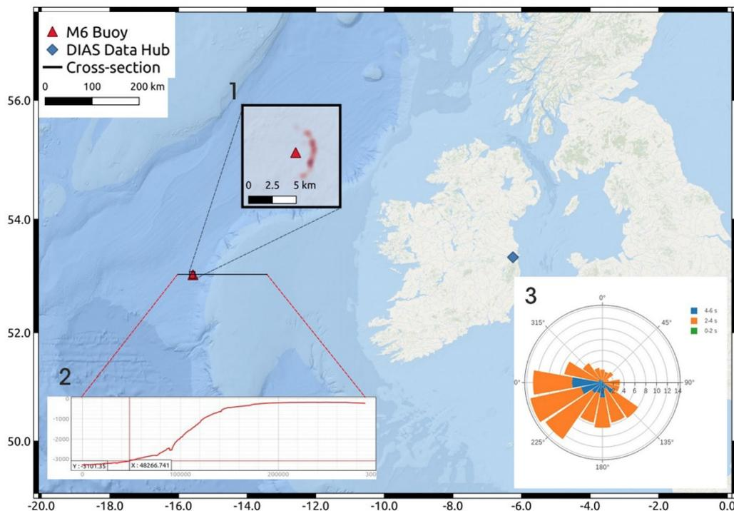
Figure 1 Map showing the positions of the M6 buoy mooring and DIAS data centre. Inset 1: Zoom of area around buoy with colour representing density of buoy location from 19/07/19 to 19/09/19. Inset 2: Depth profile along black line shown on map. Inset 3: Rose plot of daily mean wave period against wind direction
