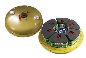
The instruments are enclosed in a pressure vessel capable of withstanding depths up to 4000m, along with lithium-
